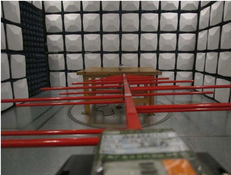
Radiated Emission View (Below 1GHz)
