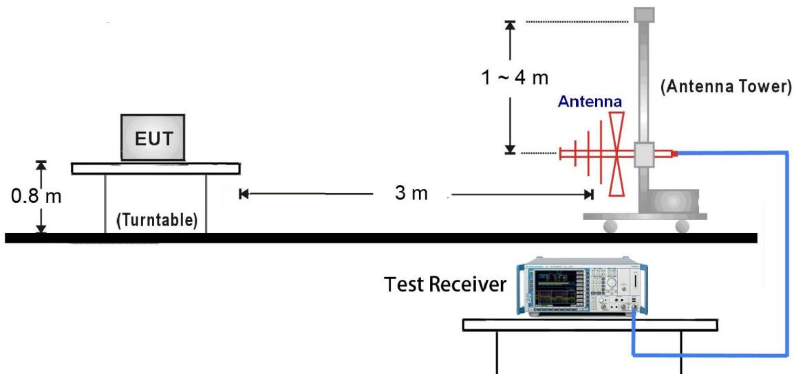
1GHz ~ 18GHz Test Setup:
