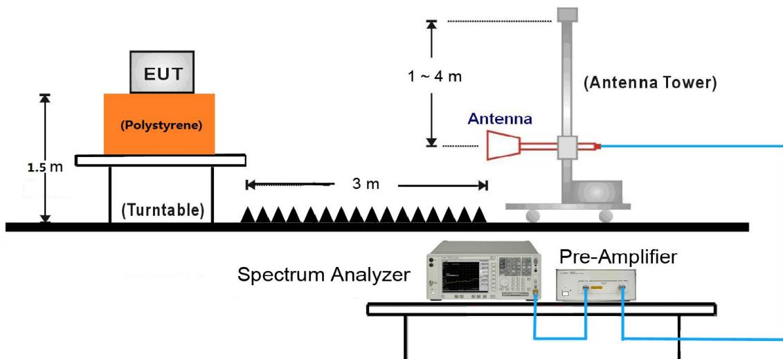
18GHz ~25GHz Test Setup:
