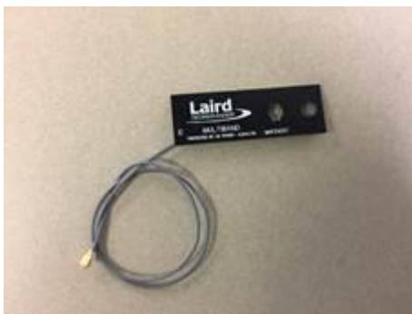
Wifi Module Antenna: It is installed on the interior of the plastic enclosure.
