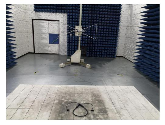
RADIATED EMISSION TEST SETUP ABOVE 1GHZ
