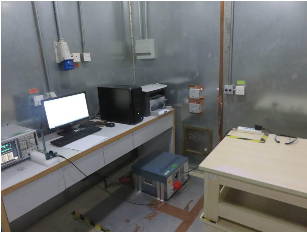
FCC RADIATED EMISSION TEST SETUP
