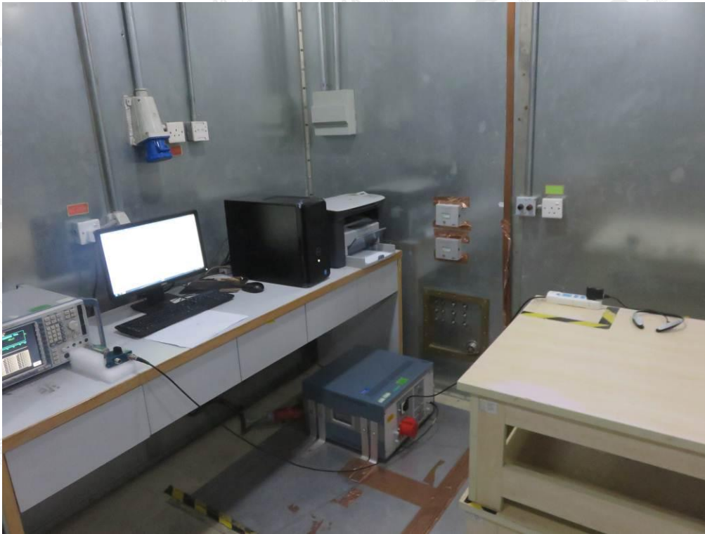
FCC RADIATED EMISSION TEST SETUP
