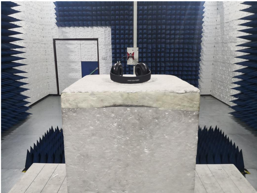
RADIATED EMISSION TEST SETUP ABOVE 1GHZ
