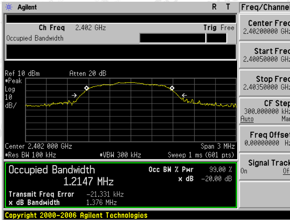
TEST PLOT OF BANDWIDTH FOR LOW CHANNEL
