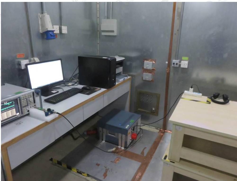
FCC RADIATED EMISSION TEST SETUP
