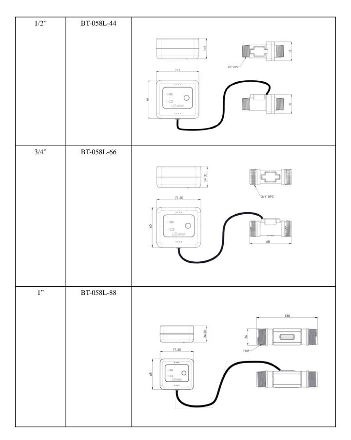
\* All of the cables and electronic devices of the flow sensors are the same. The only difference is the mechanism in size and connection.
