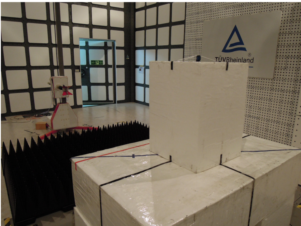
Photograph 3: Set-up for Spurious Emissions (Back View 2)
