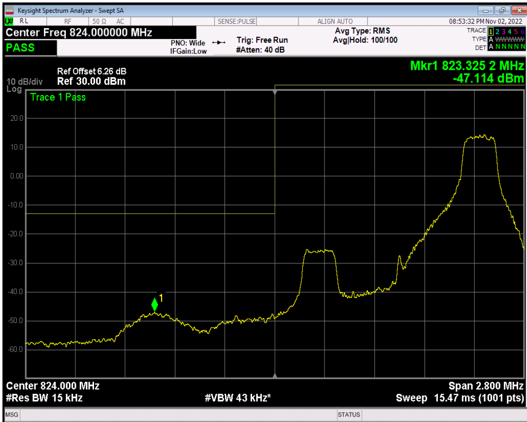
Band5 QPSK BW=1.4MHz Channel=20407 RB Size=1 Position=#Max
