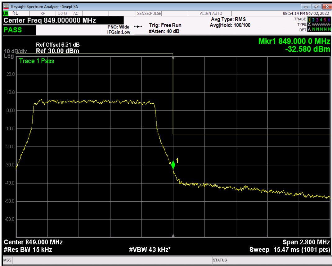
Band5 QAM16 BW=1.4MHz Channel=20643 RB Size=1 Position=#0
