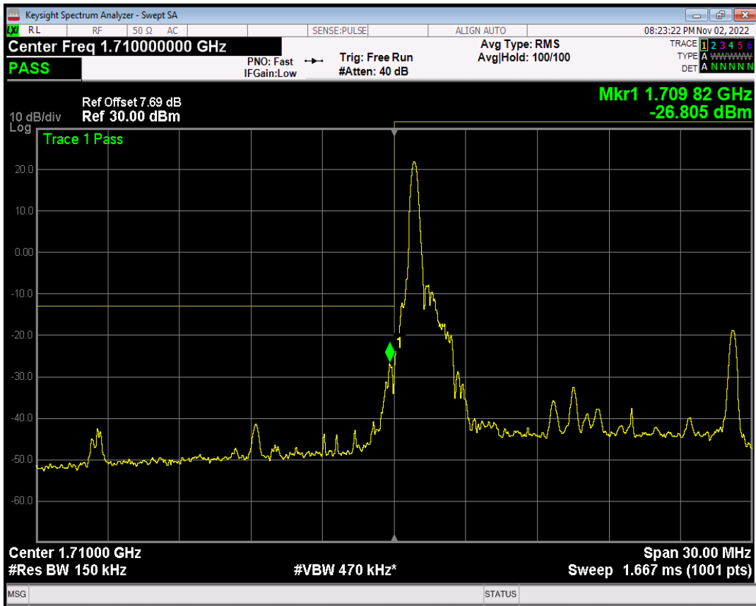
Band4 QAM16 BW=15MHz Channel=20025 RB Size=1 Position=#0
