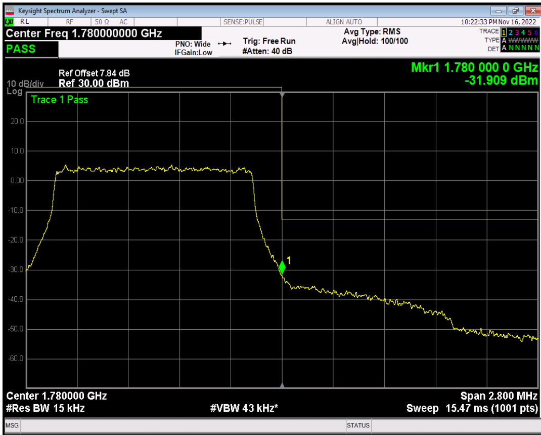
Band66 QAM16 BW=1.4MHz Channel=132665 RB Size=1 Position=#0
