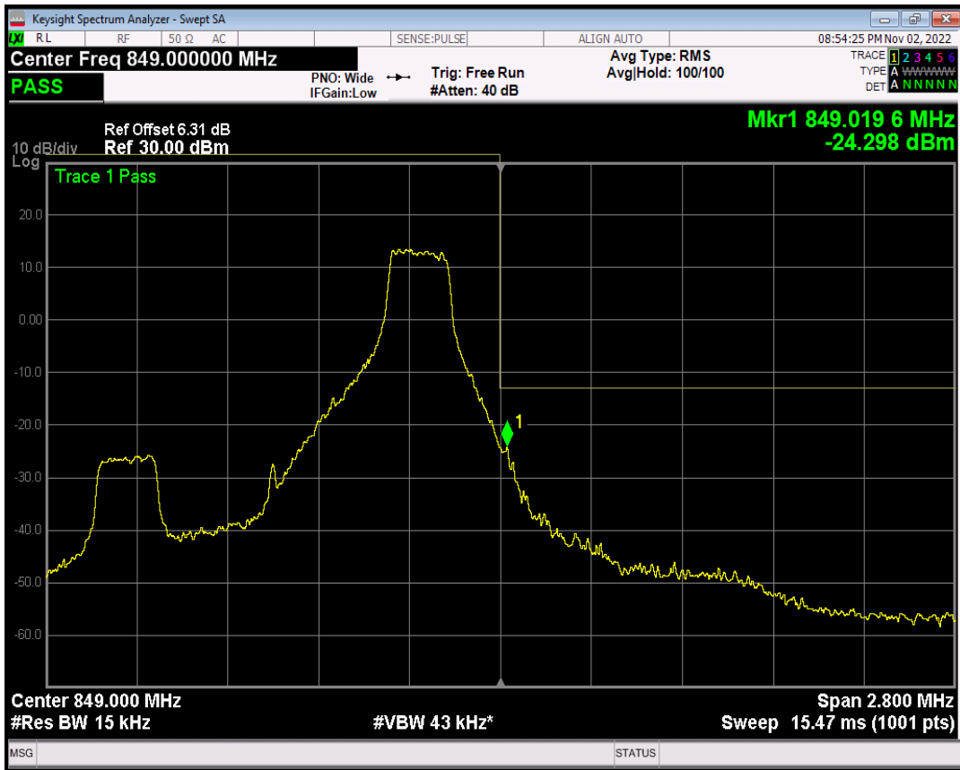
Band5 QAM16 BW=1.4MHz Channel=20643 RB Size=6 Position=#0
