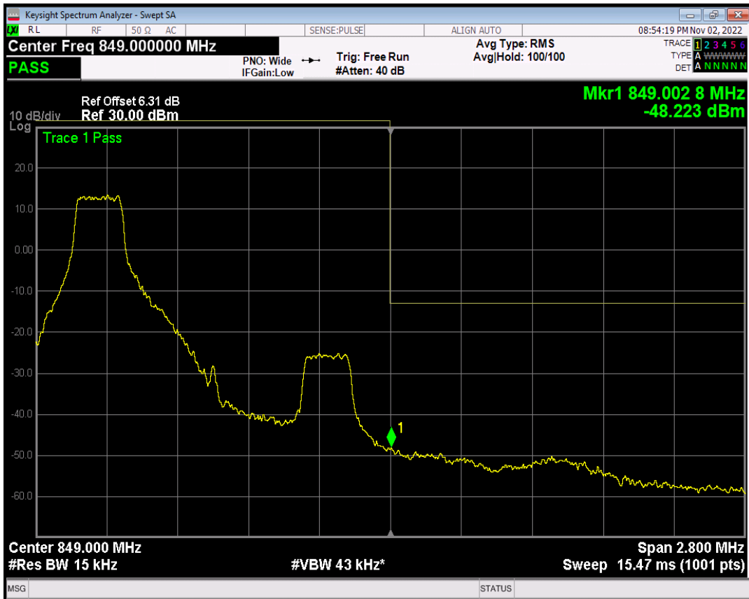
Band5 QAM16 BW=1.4MHz Channel=20643 RB Size=1 Position=#0
