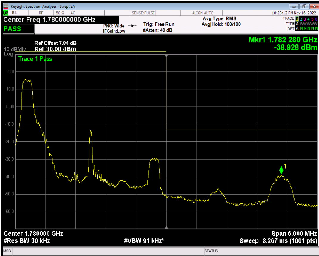
Band66 QAM16 BW=3MHz Channel=132657 RB Size=1 Position=#0
