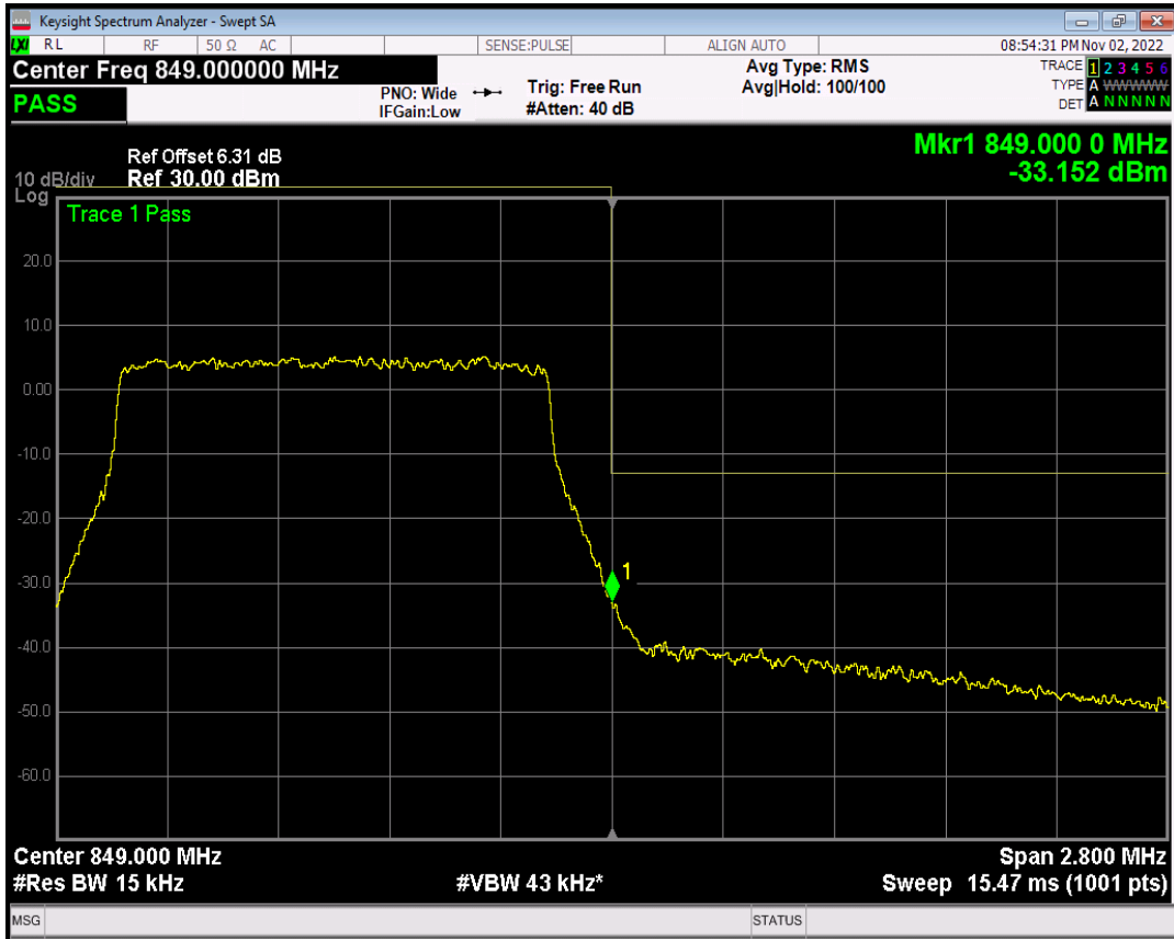
Band5 QAM16 BW=1.4MHz Channel=20643 RB Size=6 Position=#0
