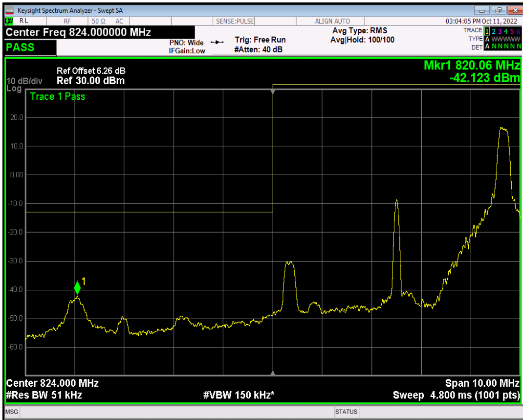
Band5 QAM16 BW=5MHz Channel=20425 RB Size=1 Position=#Max
