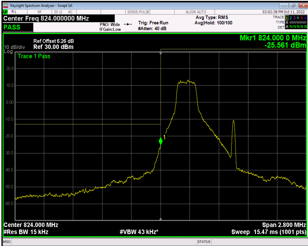
Band5 QPSK BW=1.4MHz Channel=20407 RB Size=1 Position=#0
