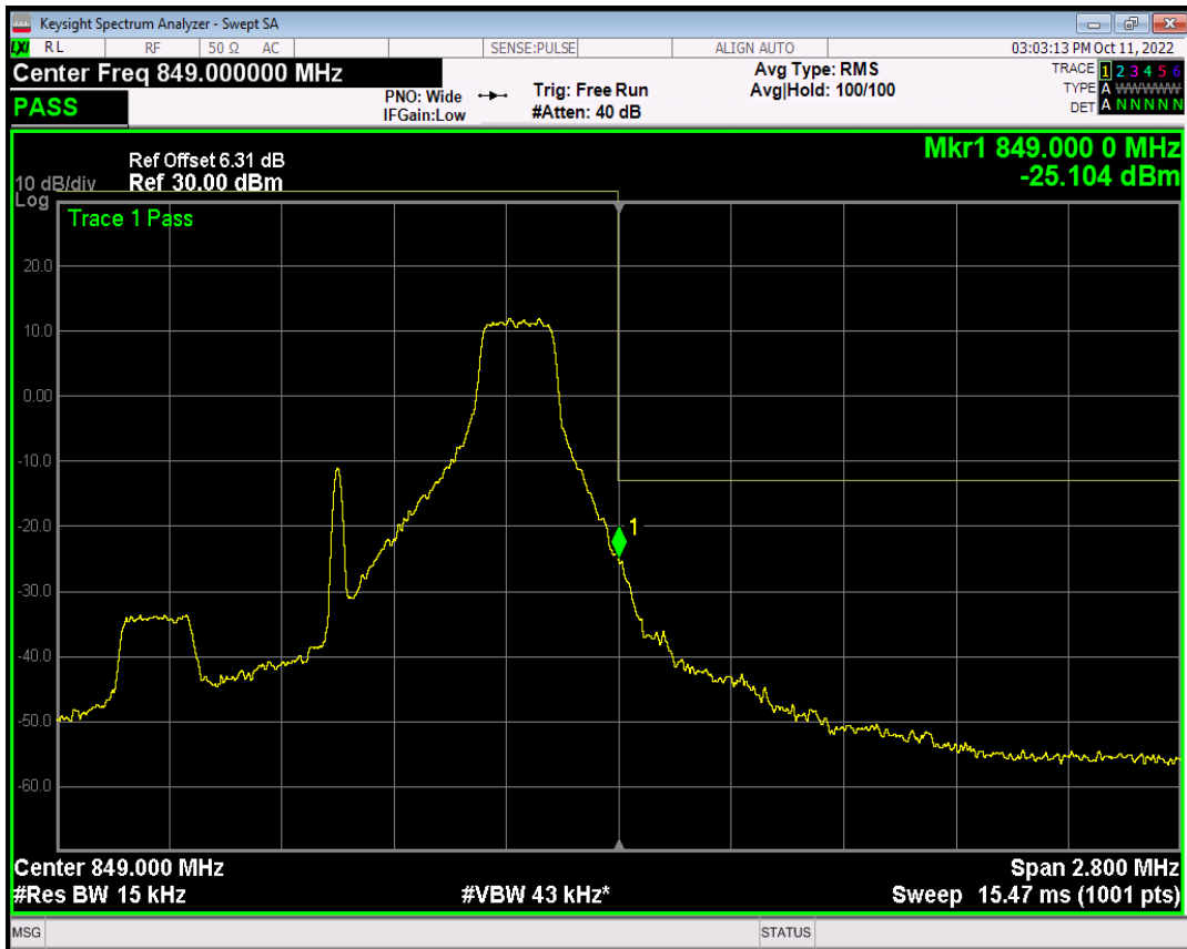
Band5 QAM16 BW=1.4MHz Channel=20643 RB Size=1 Position=#Max
