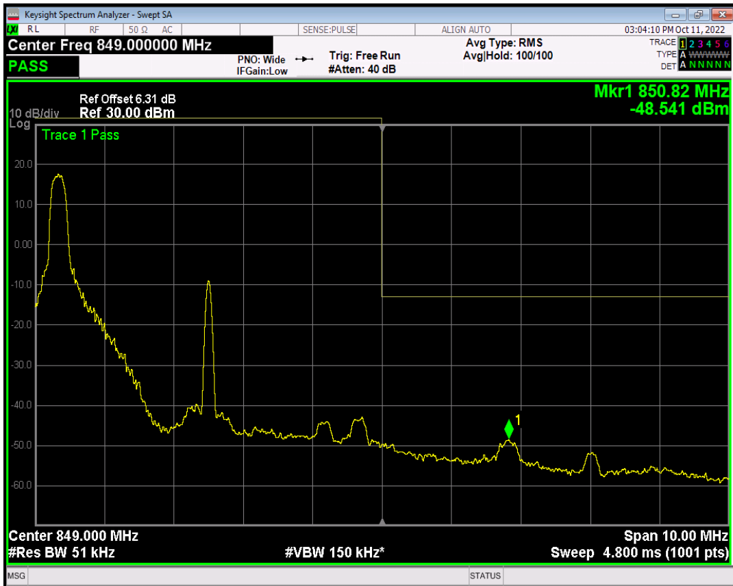
Band5 QPSK BW=5MHz Channel=20625 RB Size=1 Position=#0
