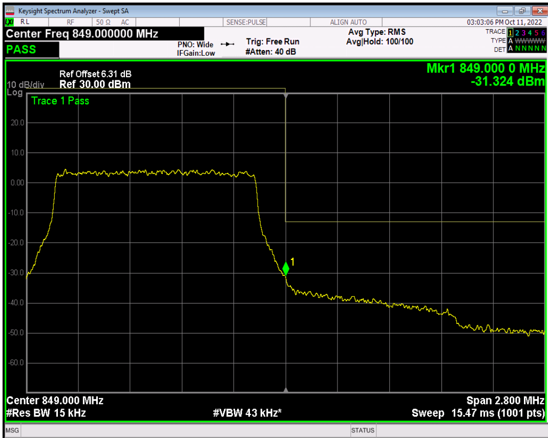
Band5 QPSK BW=1.4MHz Channel=20643 RB Size=6 Position=#0
