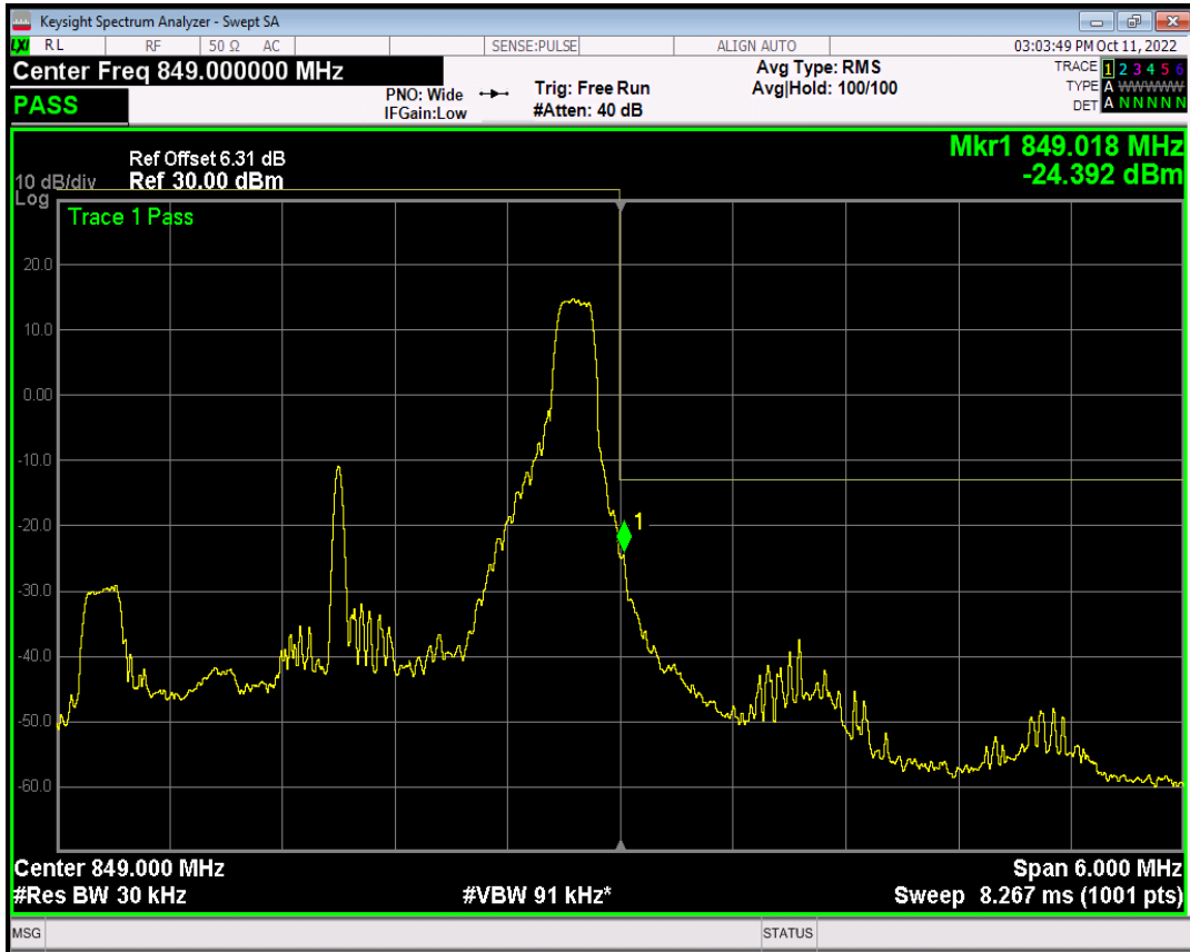
Band5 QAM16 BW=3MHz Channel=20635 RB Size=1 Position=#Max
