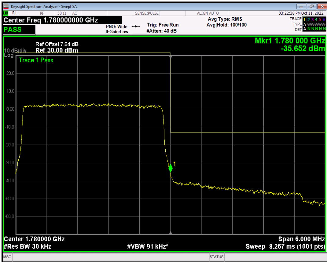
Band66 QPSK BW=3MHz Channel=132657 RB Size=15 Position=#0
