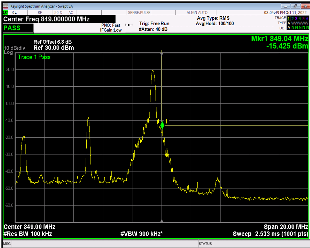
Band5 QAM16 BW=10MHz Channel=20600 RB Size=1 Position=#Max
