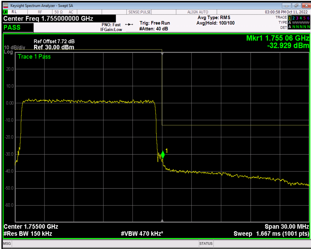
Band4 QPSK BW=20MHz Channel=20050 RB Size=1 Position=#0
