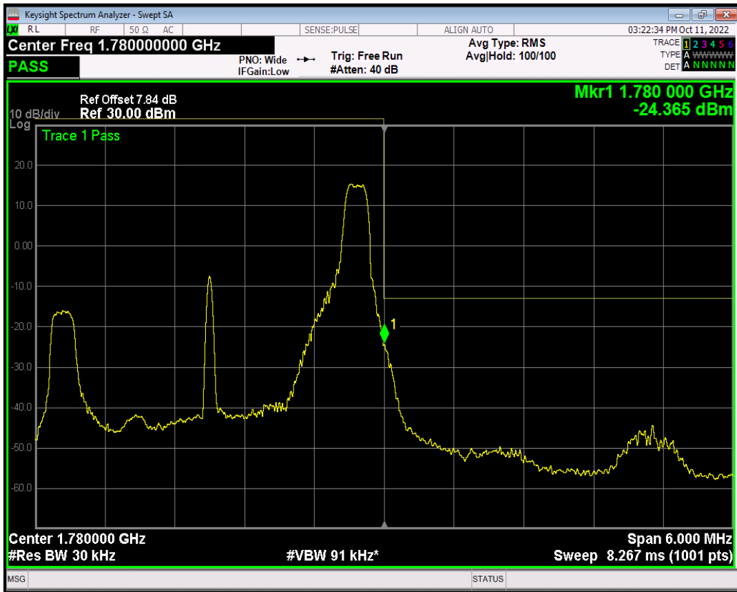
Band66 QPSK BW=3MHz Channel=132657 RB Size=15 Position=#0
