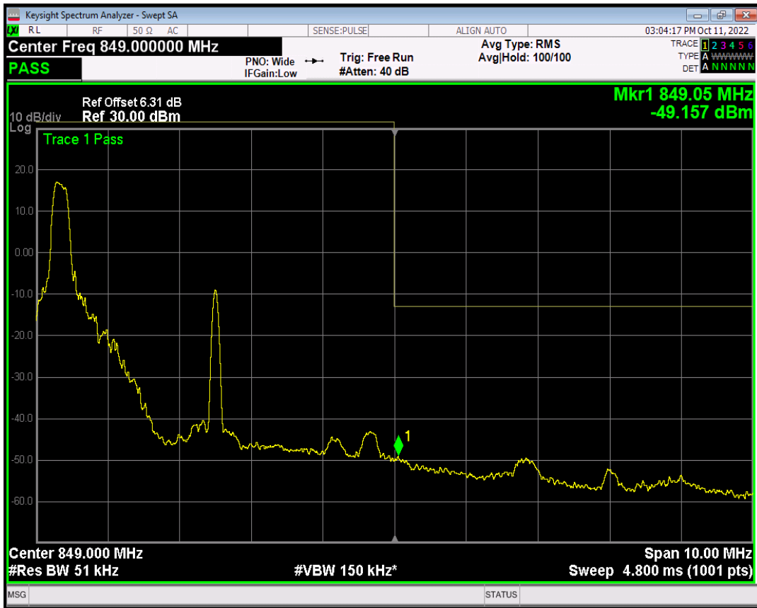
Band5 QAM16 BW=5MHz Channel=20625 RB Size=1 Position=#Max
