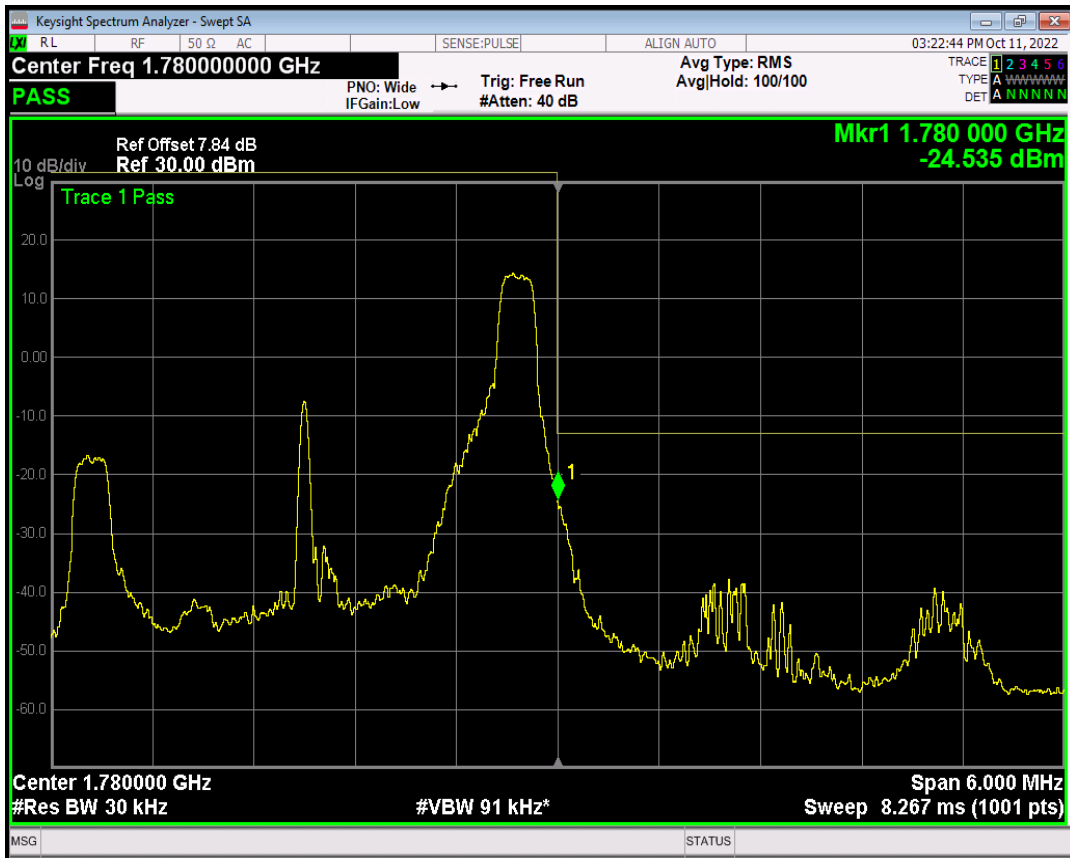
Band66 QAM16 BW=3MHz Channel=132657 RB Size=1 Position=#Max
