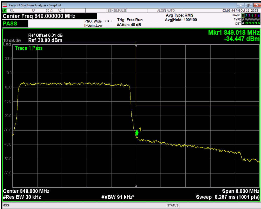
Band5 QPSK BW=3MHz Channel=20635 RB Size=15 Position=#0
