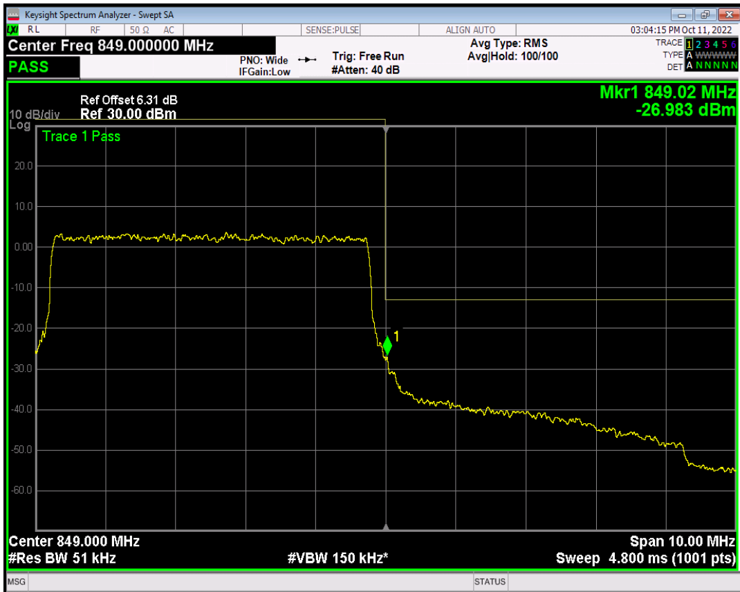
Band5 QPSK BW=5MHz Channel=20625 RB Size=25 Position=#0
