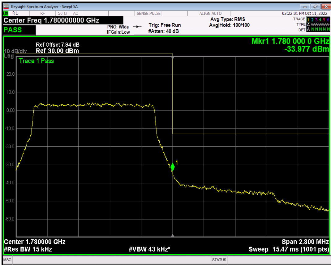
Band66 QPSK BW=1.4MHz Channel=132665 RB Size=6 Position=#0
