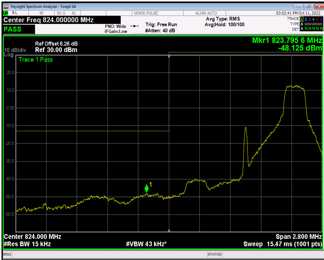
Band5 QPSK BW=1.4MHz Channel=20407 RB Size=6 Position=#0
