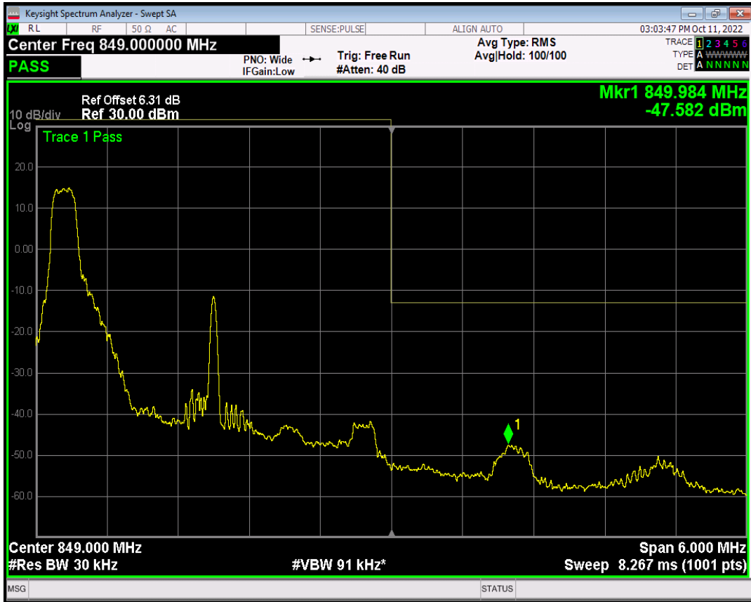
Band5 QAM16 BW=3MHz Channel=20635 RB Size=1 Position=#Max
