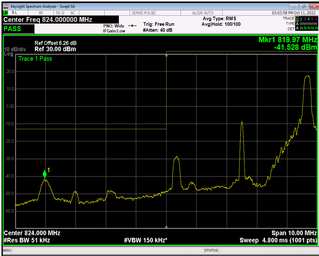
Band5 QPSK BW=5MHz Channel=20425 RB Size=25 Position=#0
