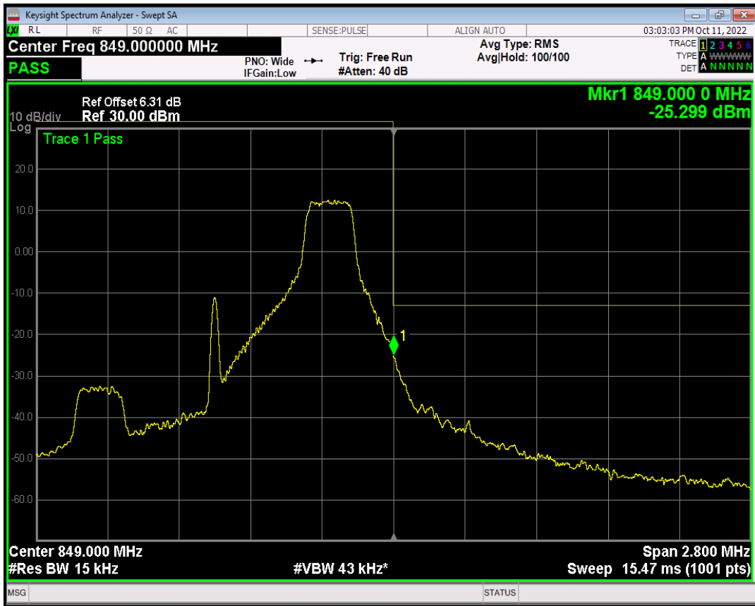
Band5 QPSK BW=1.4MHz Channel=20643 RB Size=6 Position=#0
