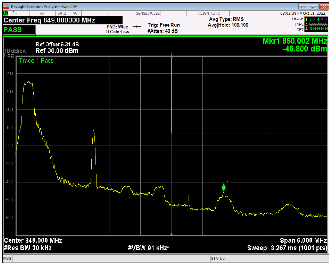
Band5 QPSK BW=3MHz Channel=20635 RB Size=1 Position=#0
