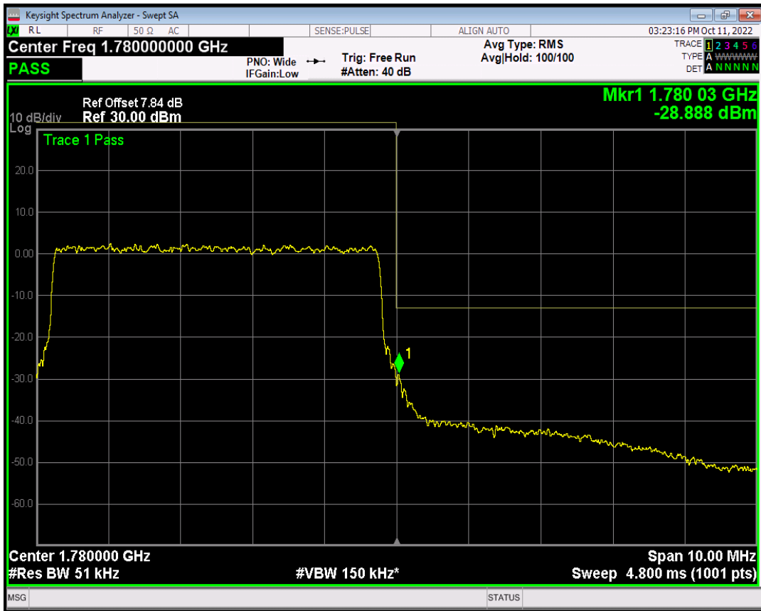
Band66 QPSK BW=10MHz Channel=132022 RB Size=1 Position=#0
