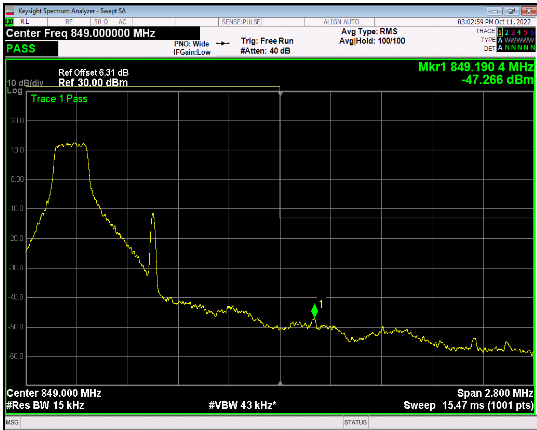
Band5 QPSK BW=1.4MHz Channel=20643 RB Size=1 Position=#0
