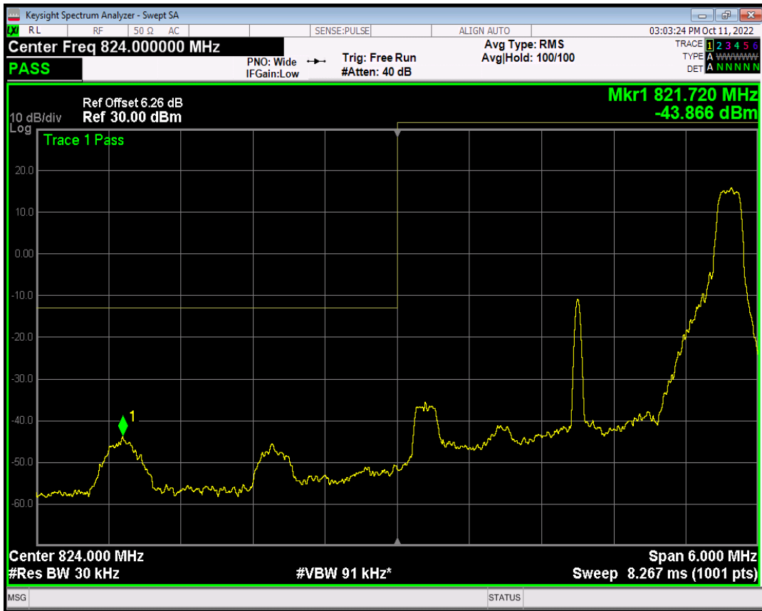
Band5 QPSK BW=3MHz Channel=20415 RB Size=15 Position=#0
