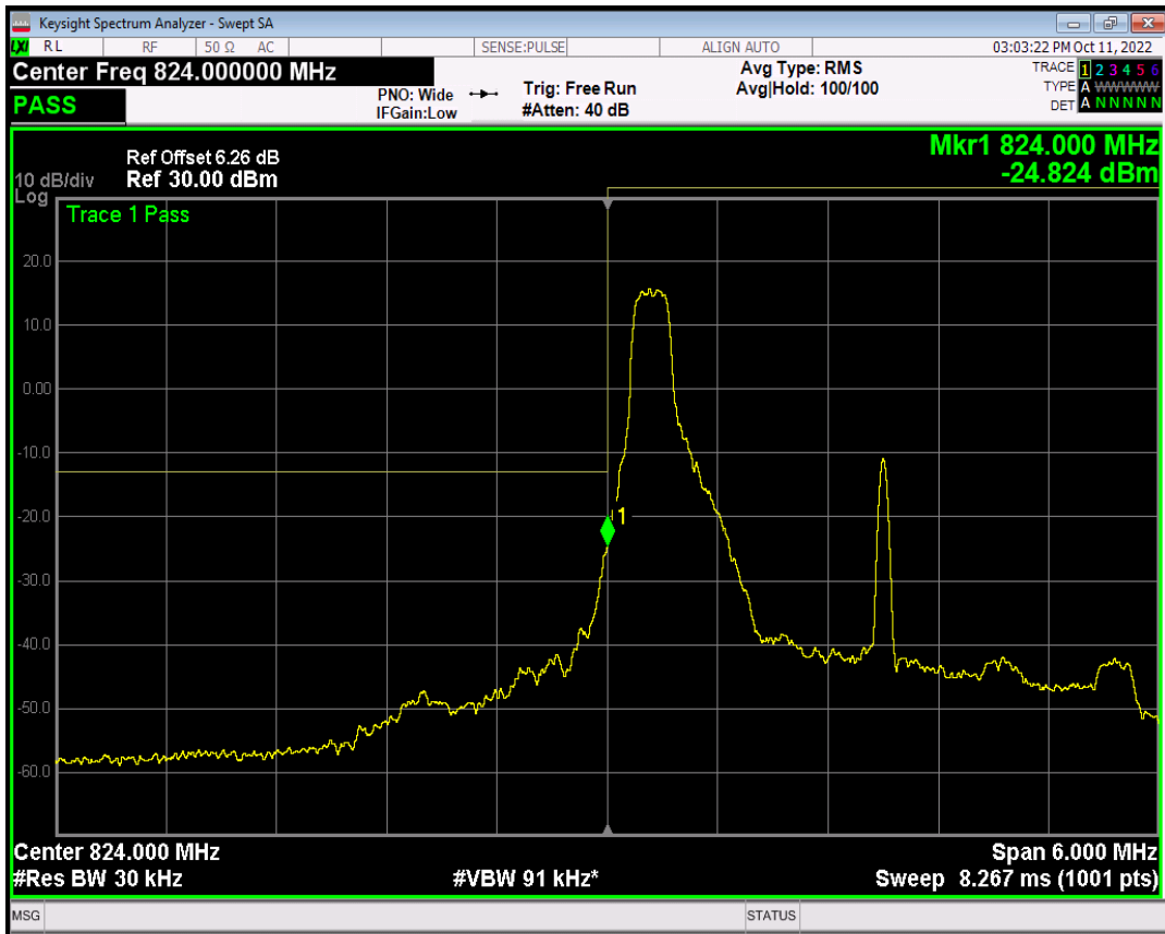
Band5 QPSK BW=3MHz Channel=20415 RB Size=1 Position=#0
