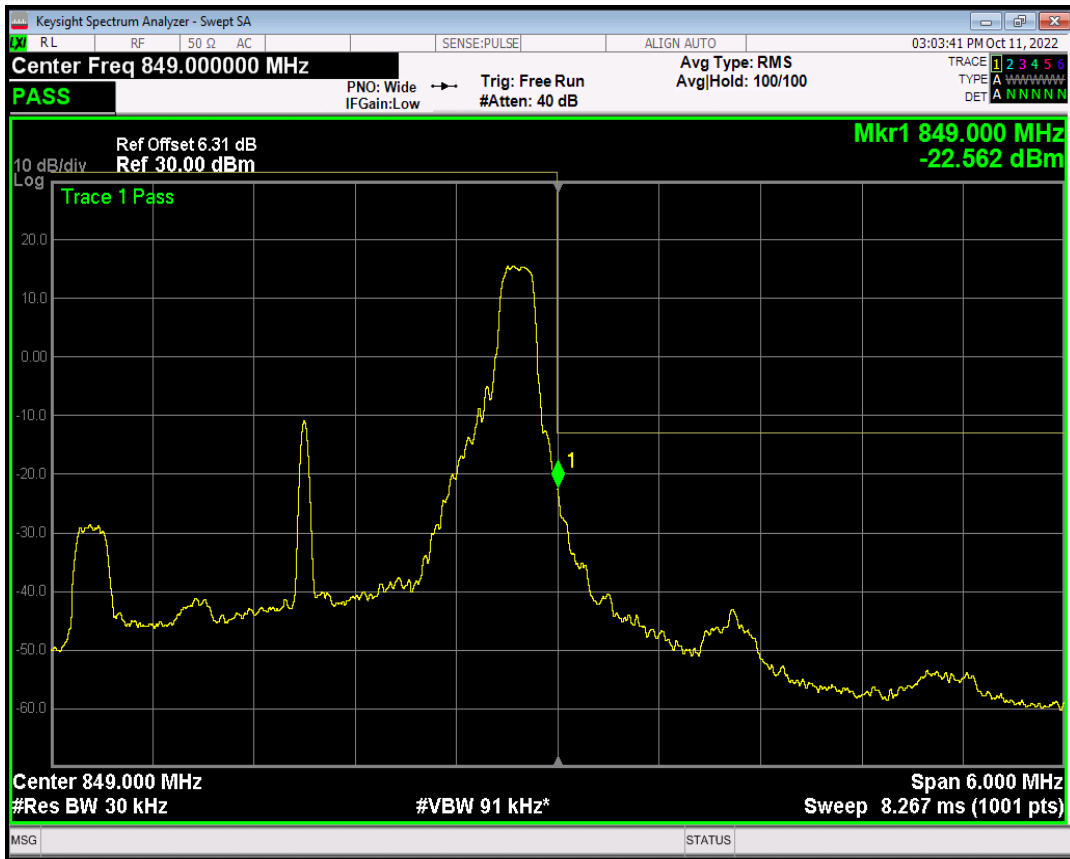
Band5 QPSK BW=3MHz Channel=20635 RB Size=15 Position=#0
