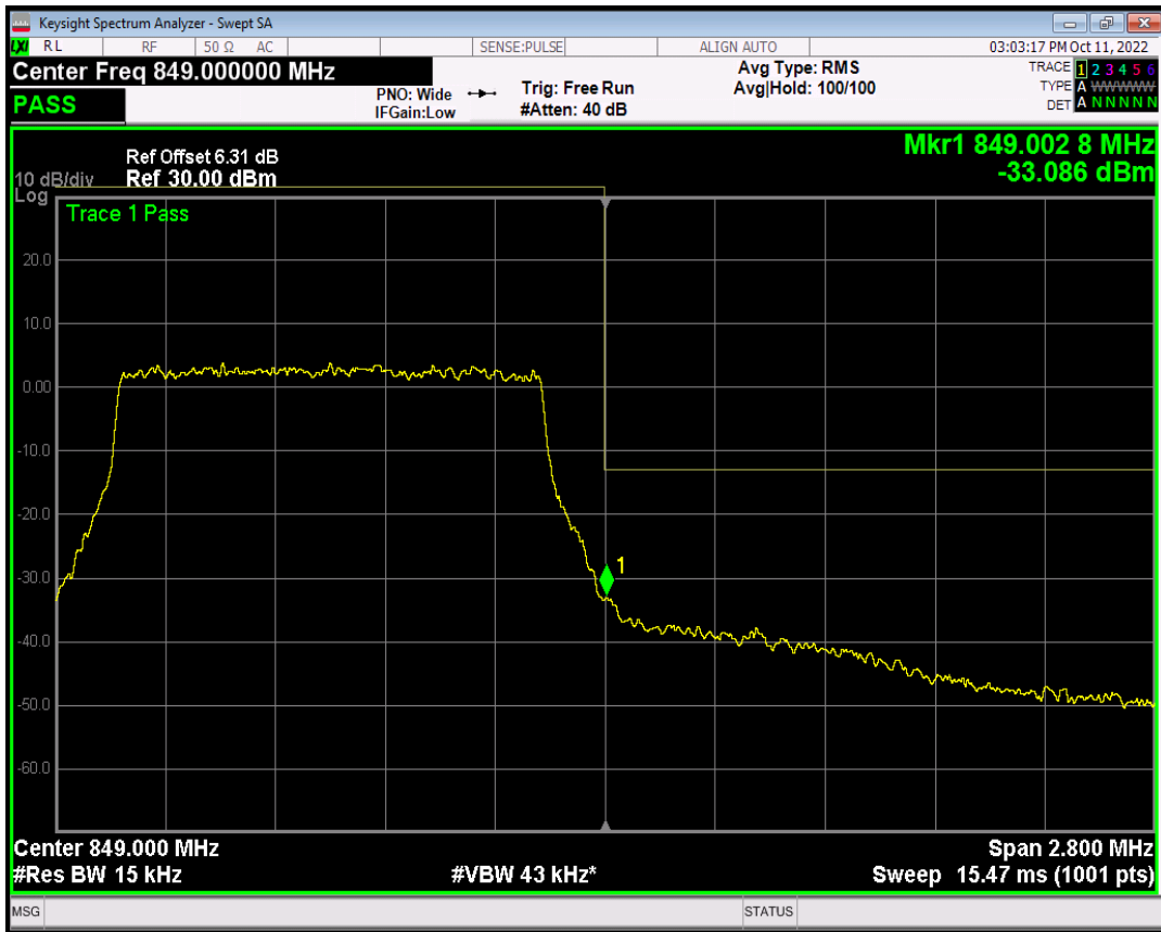
Band5 QPSK BW=3MHz Channel=20415 RB Size=1 Position=#0
