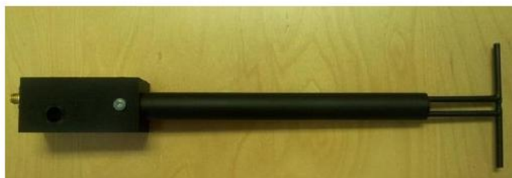
Figure 1 – MVG COMOSAR Validation Dipole
