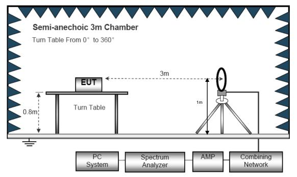
(B) Radiated Emission Test-Up Frequency 30MHz~1GHz
