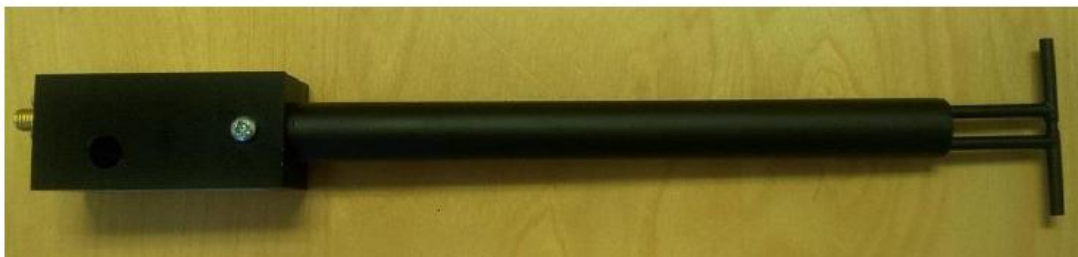
Figure 1 – MVG COMOSAR Validation Dipole
