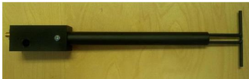
Figure 1 – MVG COMOSAR Validation Dipole
