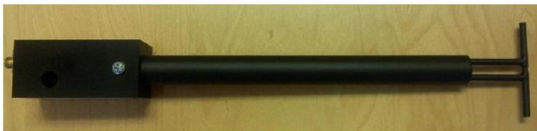
Figure 1 – MVG COMOSAR Validation Dipole
