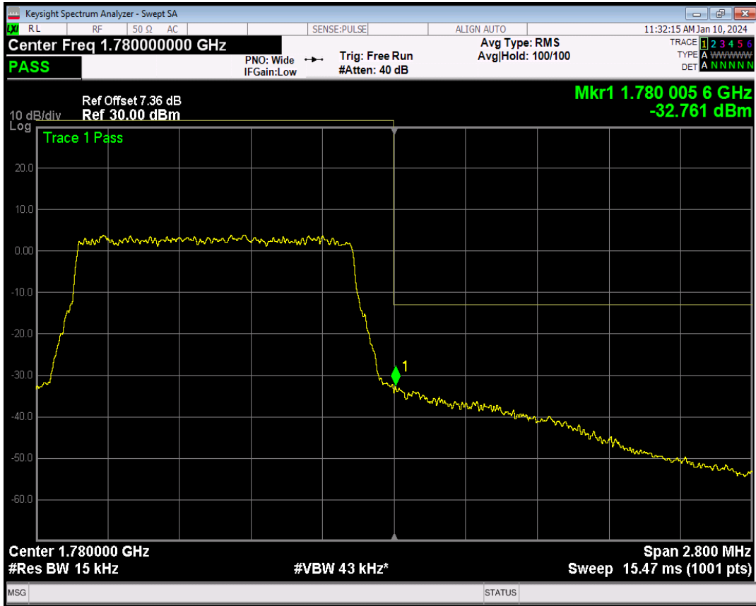
Band66 QPSK BW=3MHz Channel=131987 RB Size=1 Position=#Max
