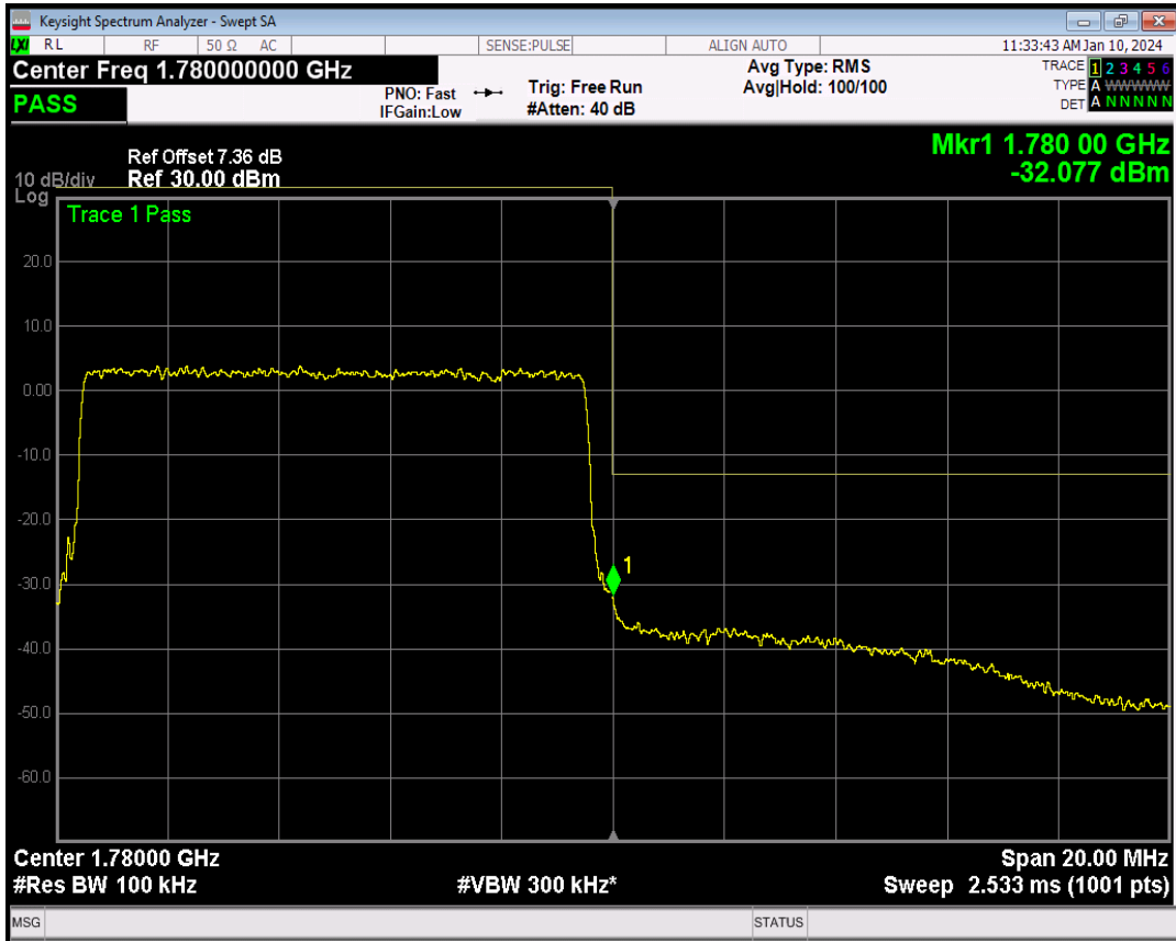
Band66 QPSK BW=10MHz Channel=132622 RB Size=50 Position=#0
