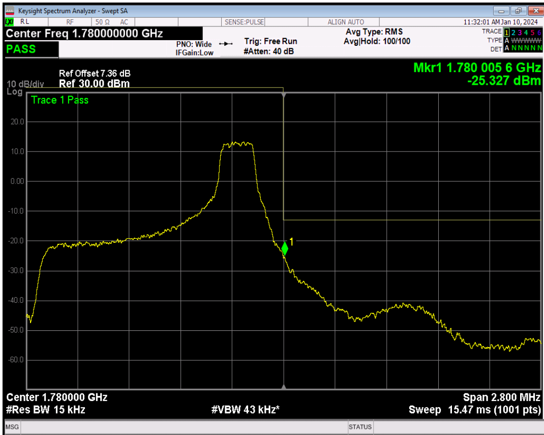
Band66 QPSK BW=1.4MHz Channel=132665 RB Size=6 Position=#0
