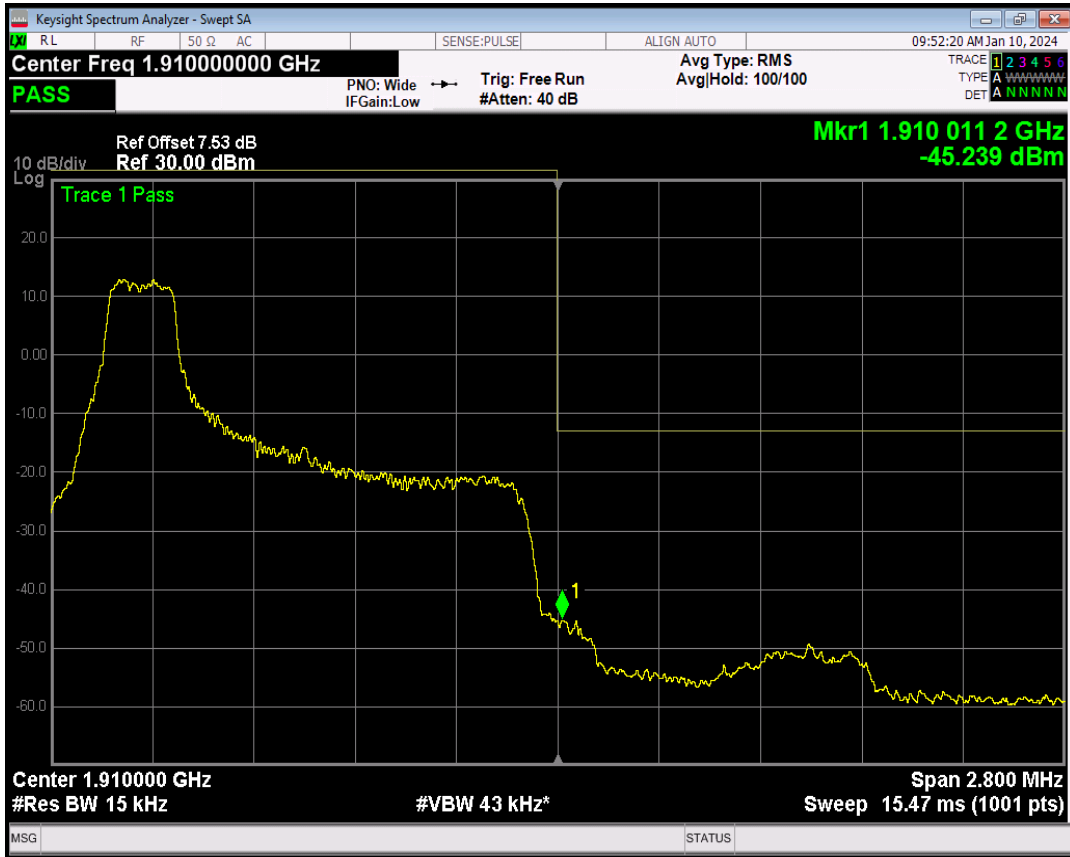
Band2 16QAM BW=1.4MHz Channel=19193 RB Size=1 Position=#Max
