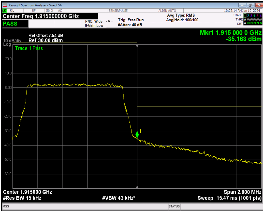
Band25 QPSK BW=3MHz Channel=26055 RB Size=1 Position=#0
