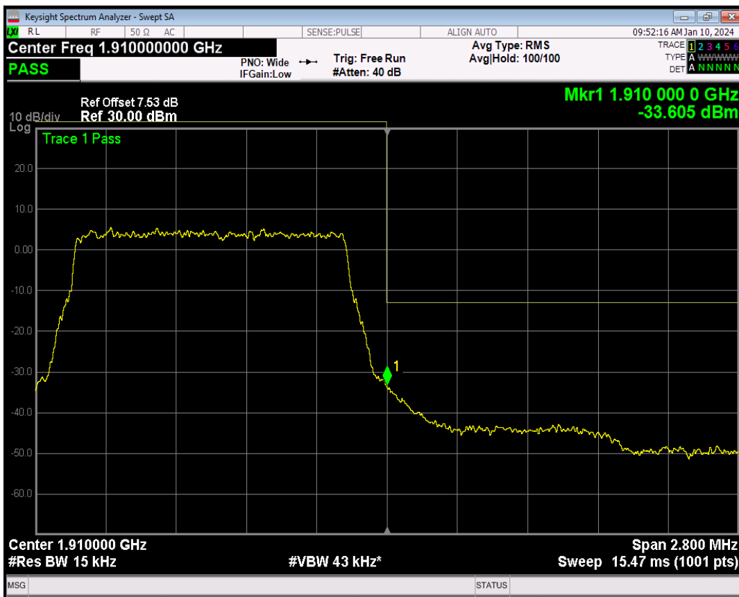
Band2 QPSK BW=1.4MHz Channel=19193 RB Size=6 Position=#0
