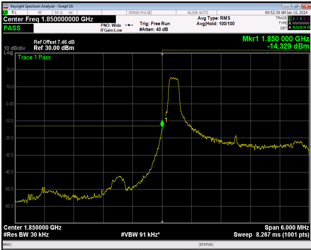
Band2 16QAM BW=3MHz Channel=18615 RB Size=1 Position=#Max
