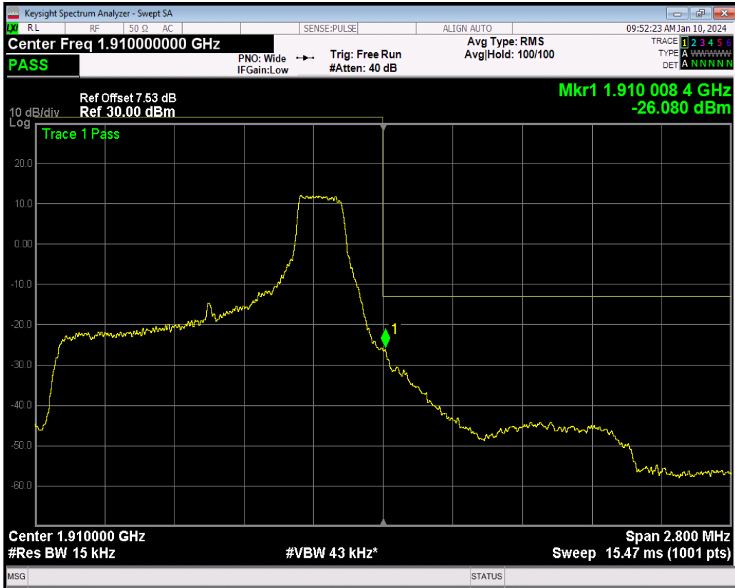
Band2 16QAM BW=1.4MHz Channel=19193 RB Size=1 Position=#Max
