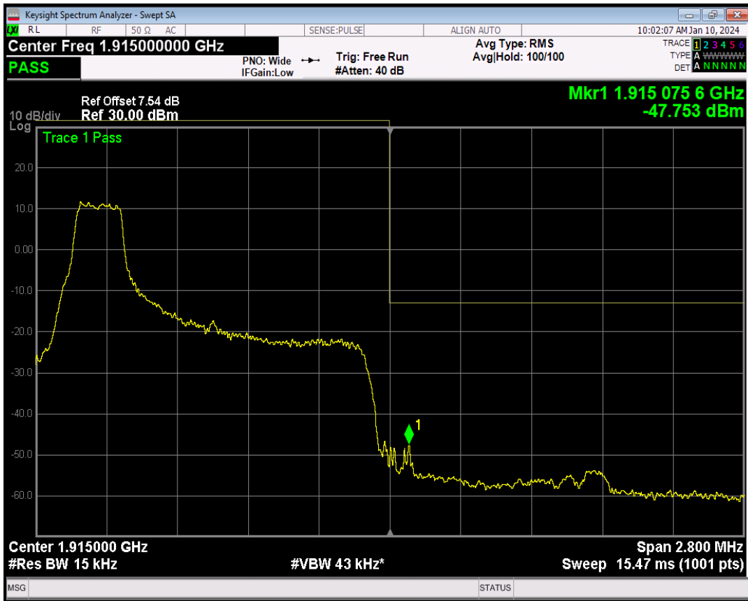
Band25 16QAM BW=1.4MHz Channel=26683 RB Size=1 Position=#Max
