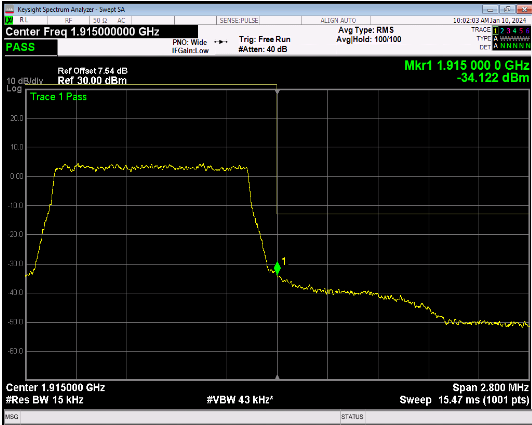
Band25 QPSK BW=1.4MHz Channel=26683 RB Size=6 Position=#0
