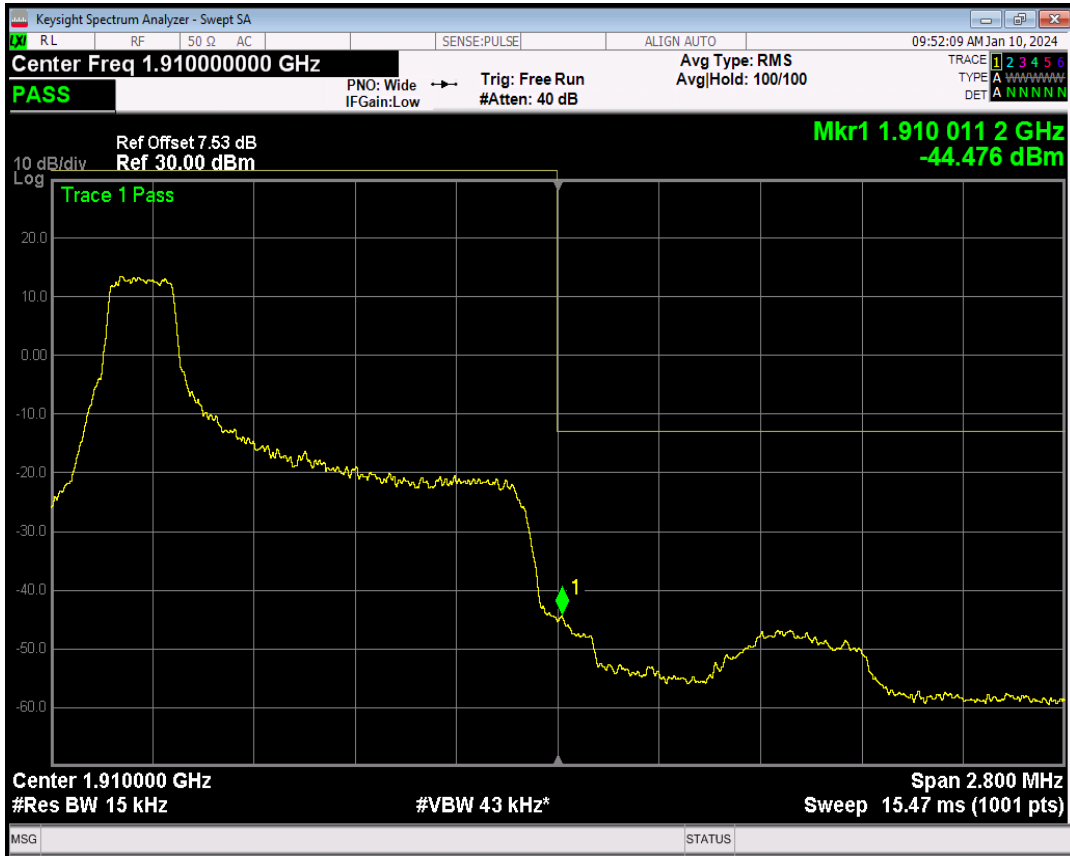
Band2 QPSK BW=1.4MHz Channel=19193 RB Size=1 Position=#0
