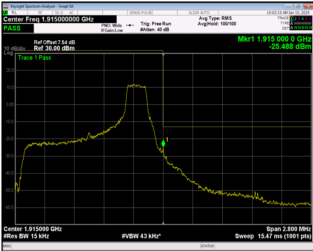
Band25 16QAM BW=1.4MHz Channel=26683 RB Size=1 Position=#Max
