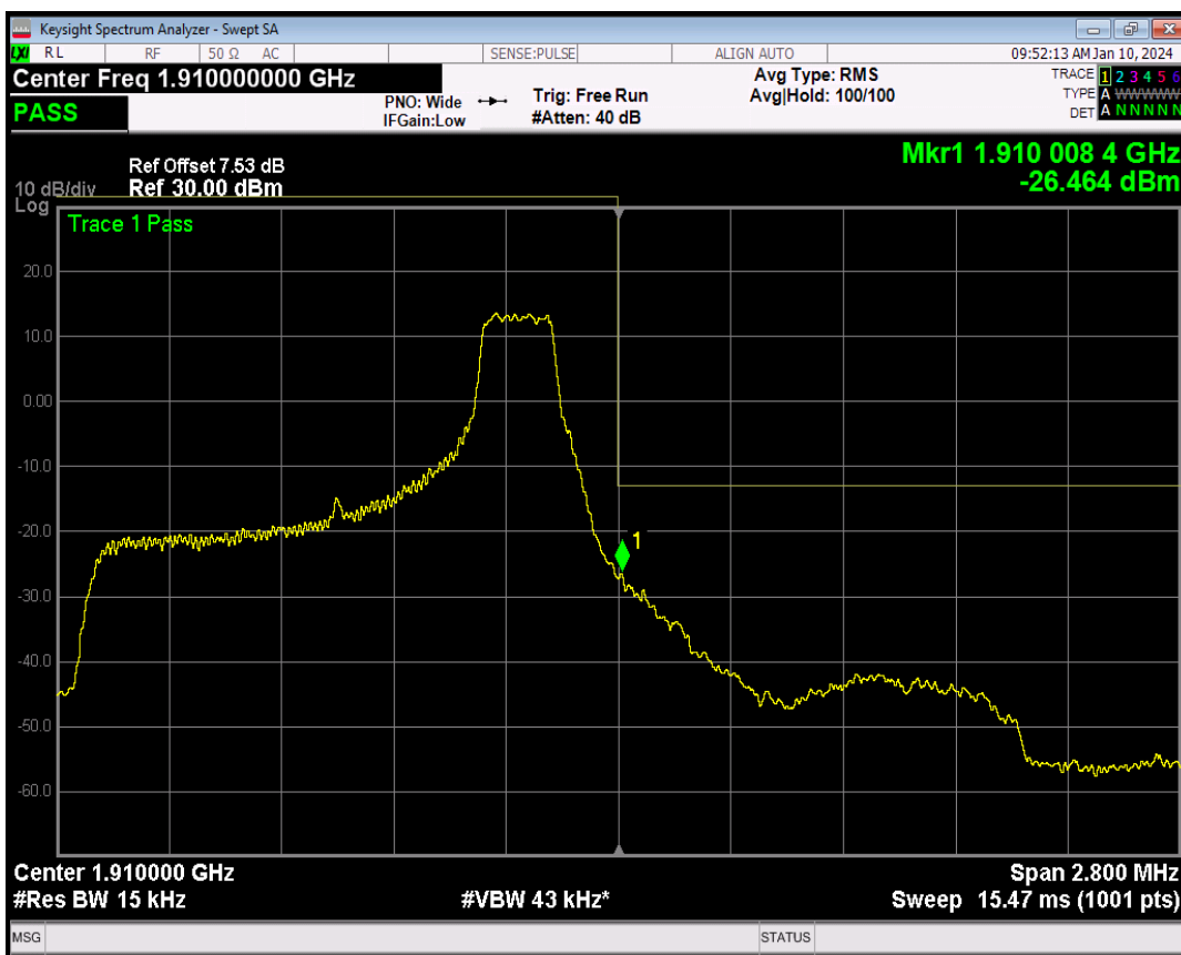
Band2 QPSK BW=1.4MHz Channel=19193 RB Size=6 Position=#0
