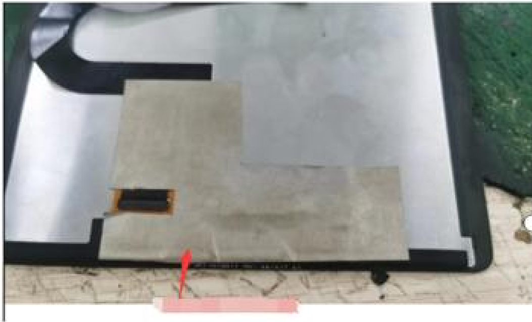
Shielding of screen cables with conductive cloth
