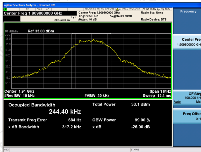
26dB&99% Occupied Bandwidth Plot on Channel 810
