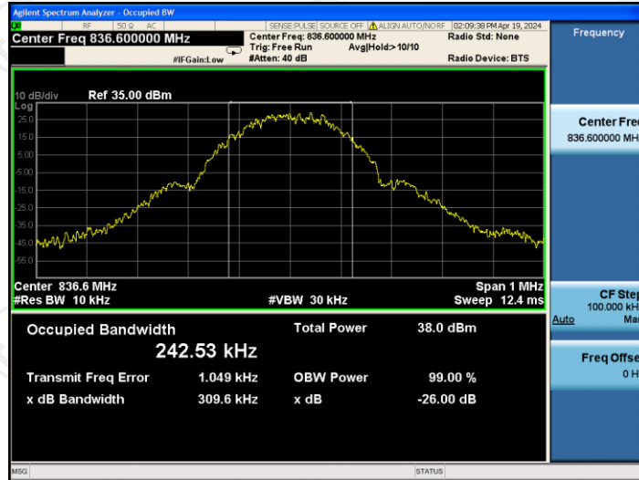
26dB&99% Occupied Bandwidth Plot on Channel 251
