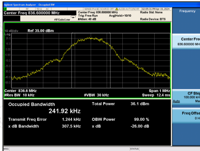
26dB&99% Occupied Bandwidth Plot on Channel 251
