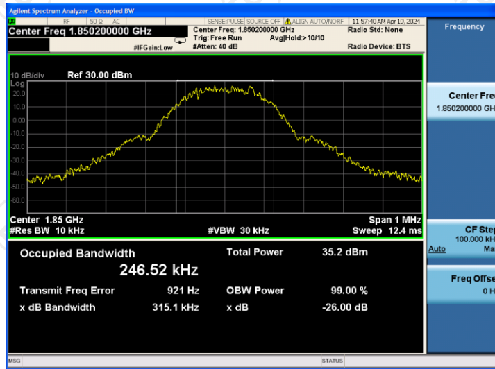
26dB&99% Occupied Bandwidth Plot on Channel 661
