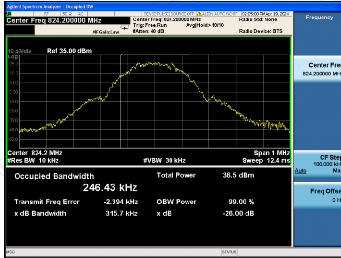
26dB&99% Occupied Bandwidth Plot on Channel 190
