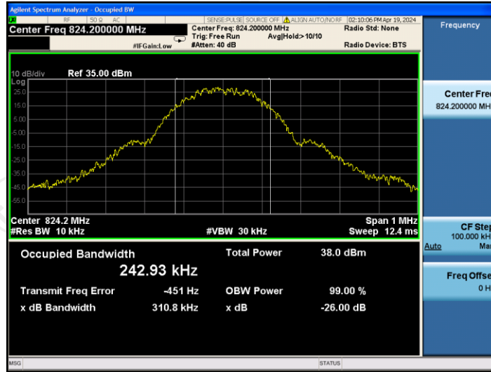
26dB&99% Occupied Bandwidth Plot on Channel 190
