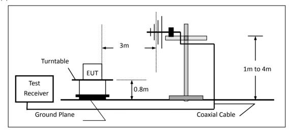
(c) For radiated emissions above 1000MHz
