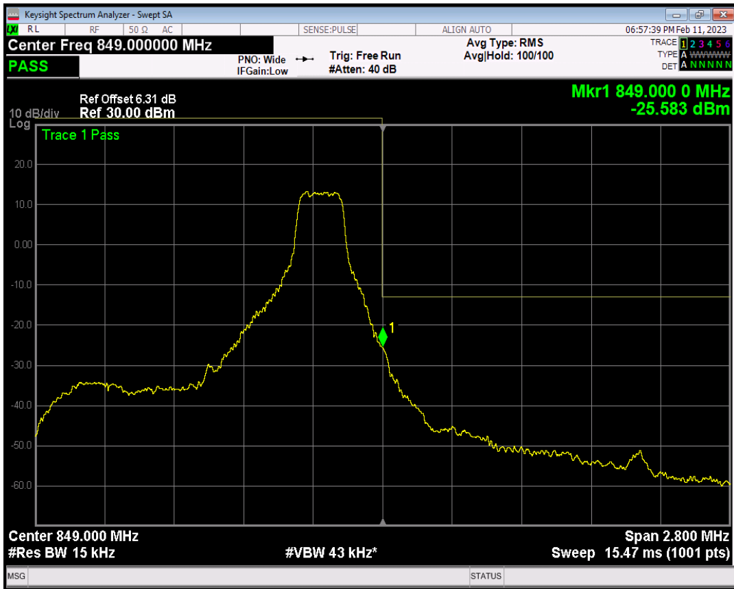
Band5 QPSK BW=1.4MHz Channel=20643 RB Size=6 Position=#0
