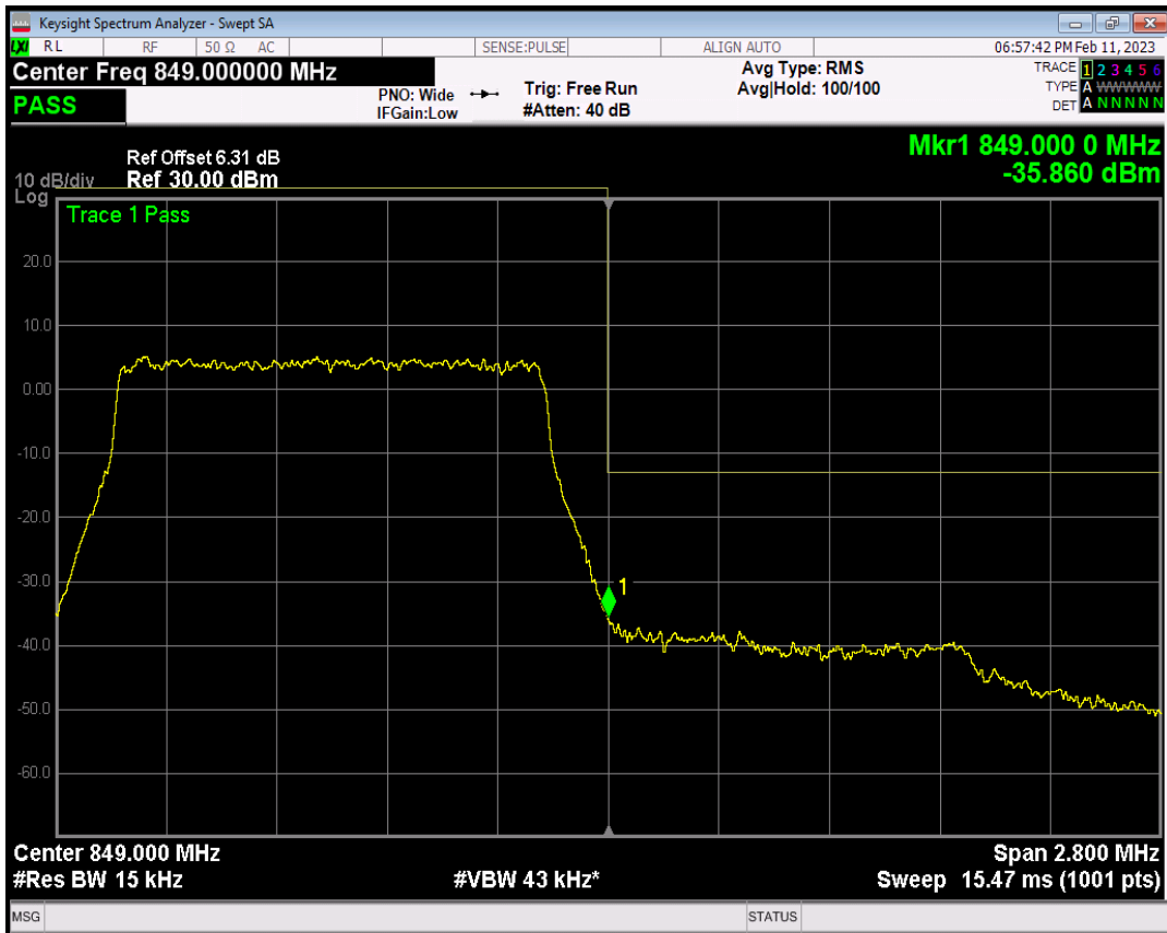
Band5 QPSK BW=1.4MHz Channel=20643 RB Size=6 Position=#0
