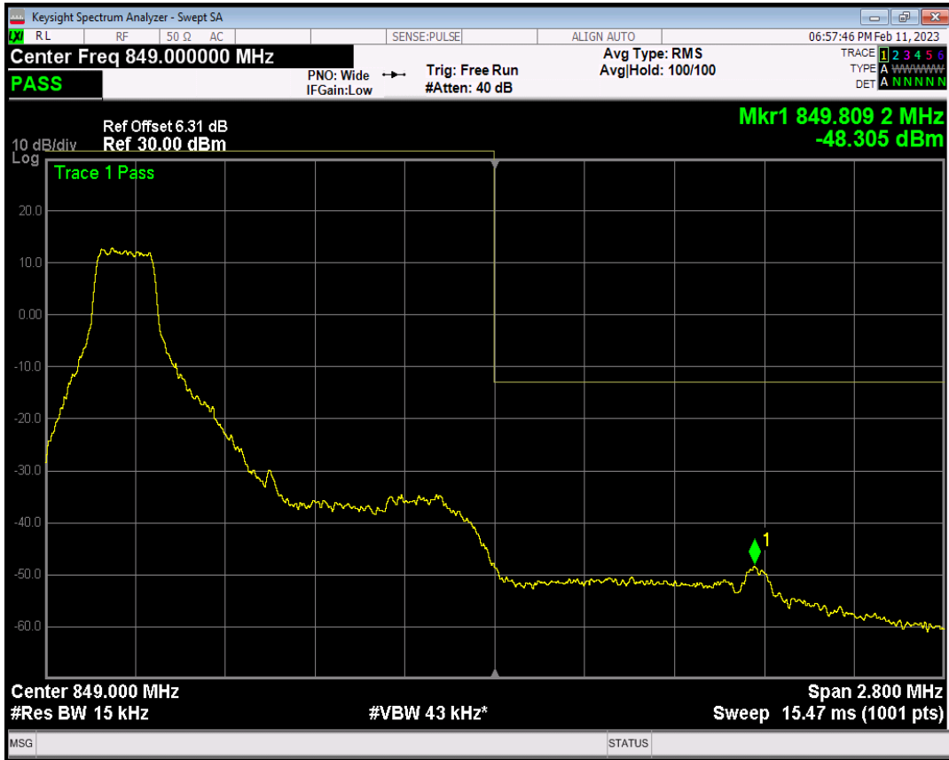
Band5 QAM16 BW=1.4MHz Channel=20643 RB Size=1 Position=#Max
