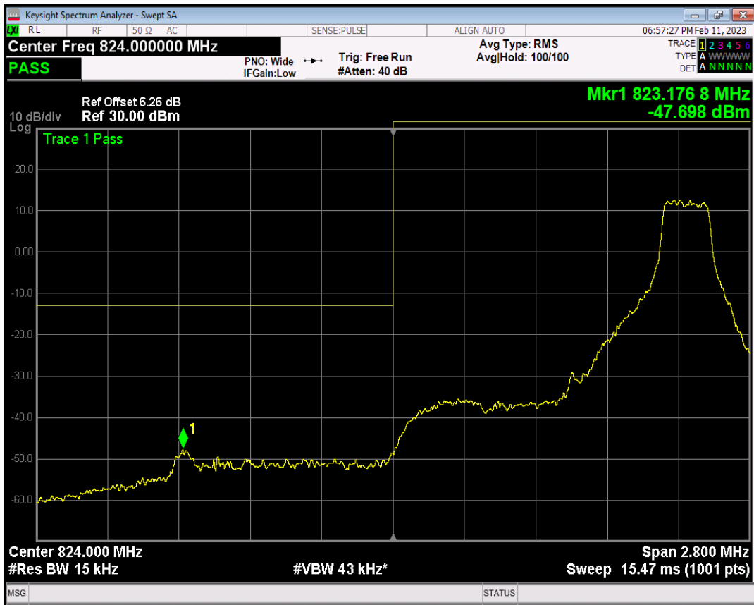
Band5 QAM16 BW=1.4MHz Channel=20407 RB Size=1 Position=#Max
