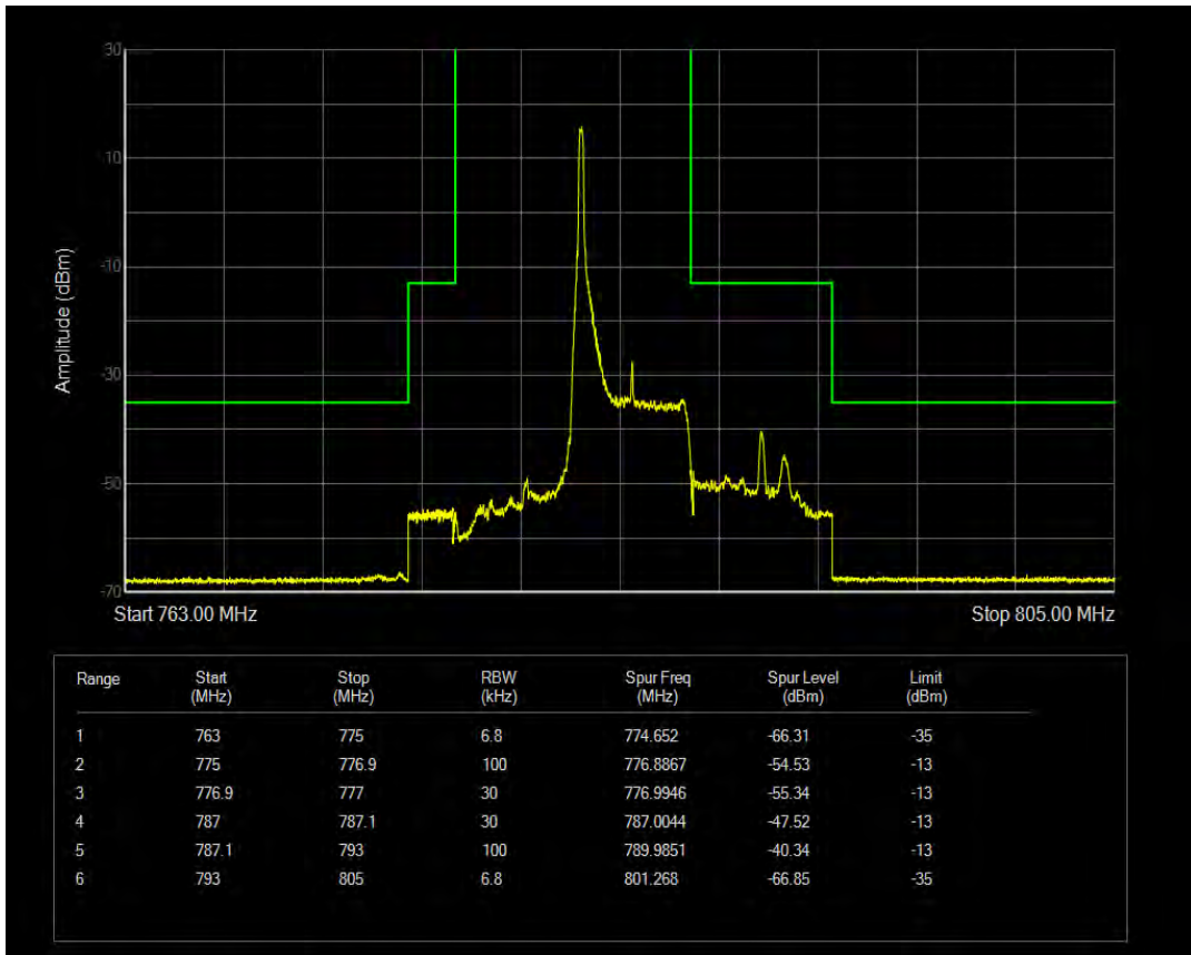
Band13 QPSK BW=5MHz Channel=23255 RB Size=1 Position=#0
