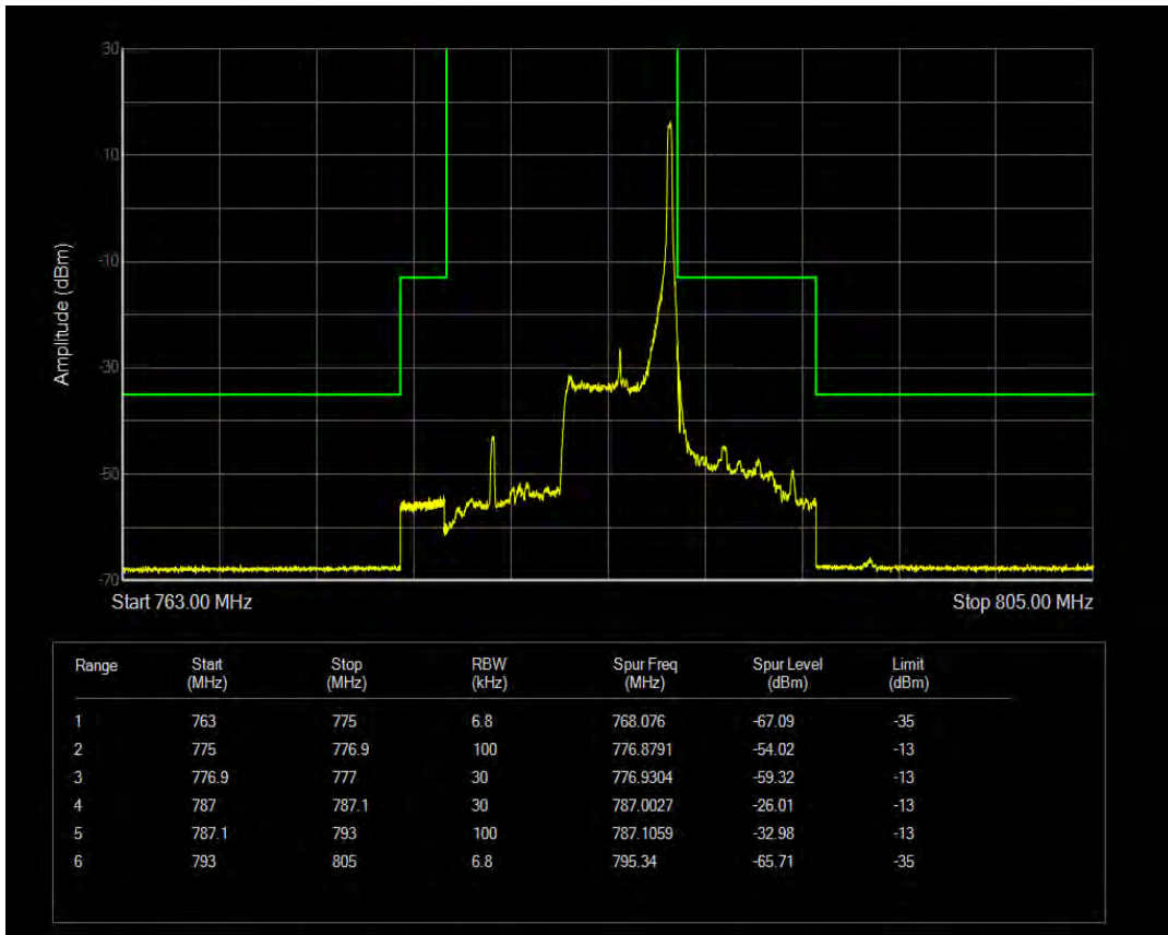
Band13 QPSK BW=5MHz Channel=23255 RB Size=25 Position=#0
