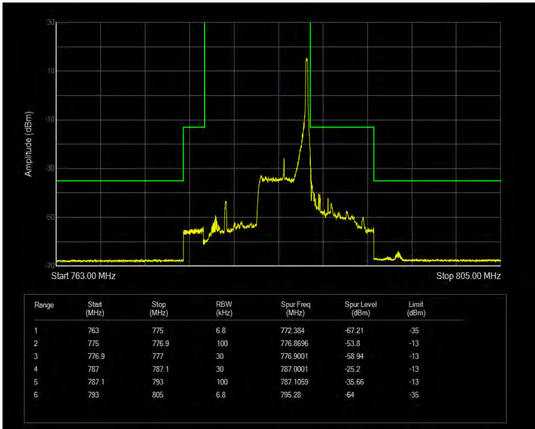
Band13 QAM16 BW=5MHz Channel=23255 RB Size=1 Position=#Max
