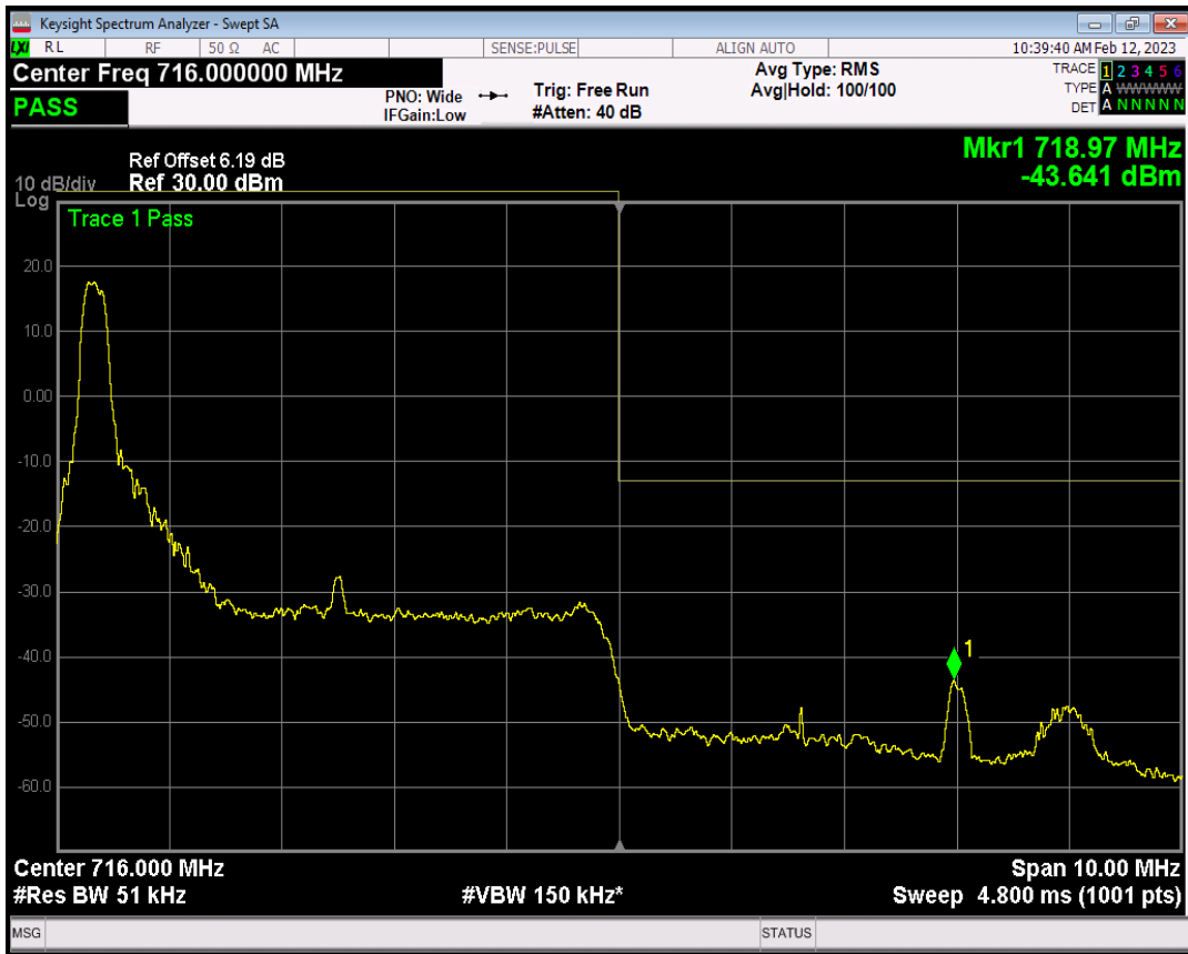
Band17 QAM16 BW=5MHz Channel=23825 RB Size=1 Position=#Max
