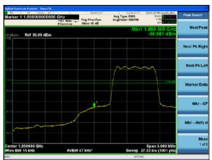
Conducted Band Edge plot on channel 1175
