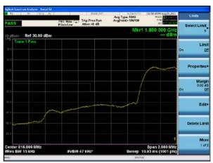
Conducted Band Edge plot on channel 670
