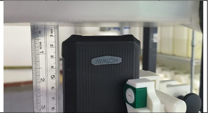
Bottom Side (Separation distance of 10mm)
