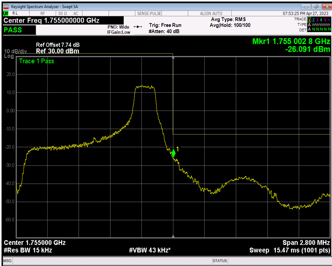
Band4 16QAM BW=1.4MHz Channel=20393 RB Size=1 Position=#Max
