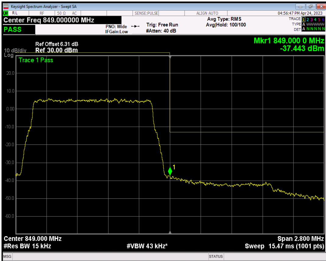
Band5 QPSK BW=1.4MHz Channel=20643 RB Size=6 Position=#0
