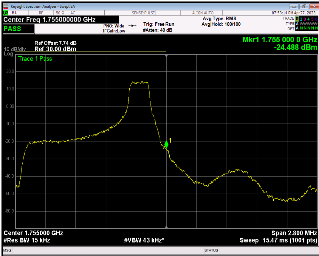
Band4 QPSK BW=1.4MHz Channel=20393 RB Size=6 Position=#0
