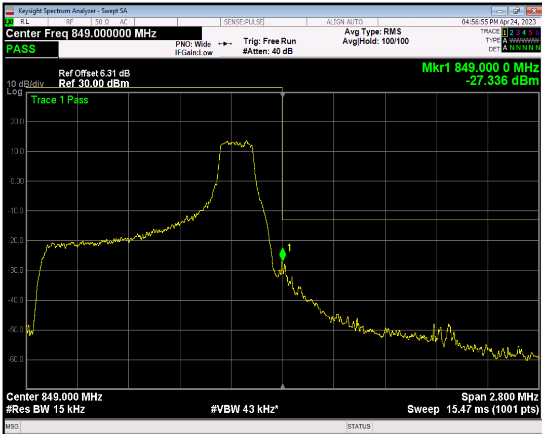
Band5 16QAM BW=1.4MHz Channel=20643 RB Size=1 Position=#Max
