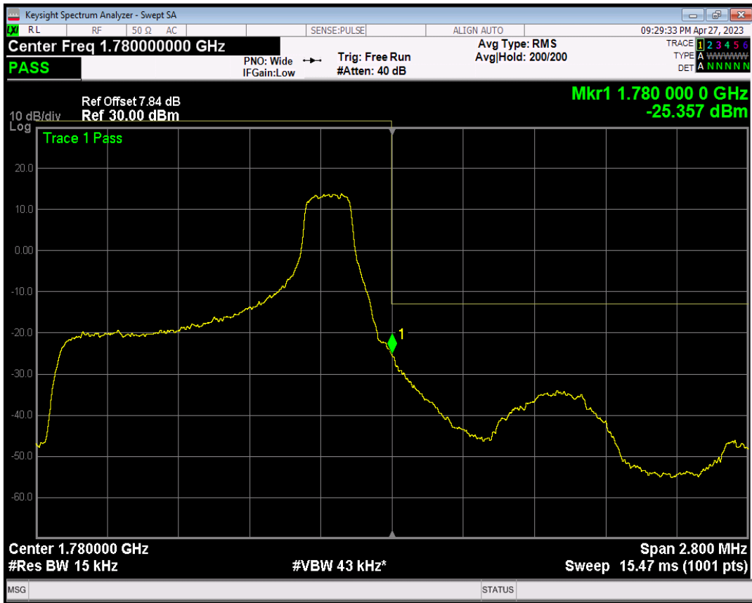
Band66 QPSK BW=1.4MHz Channel=132665 RB Size=6 Position=#0
