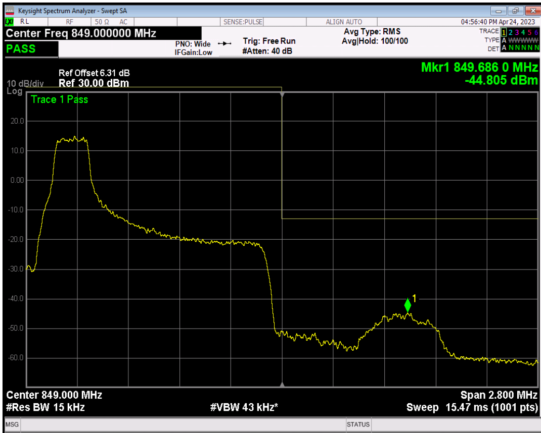
Band5 QPSK BW=1.4MHz Channel=20643 RB Size=1 Position=#0
