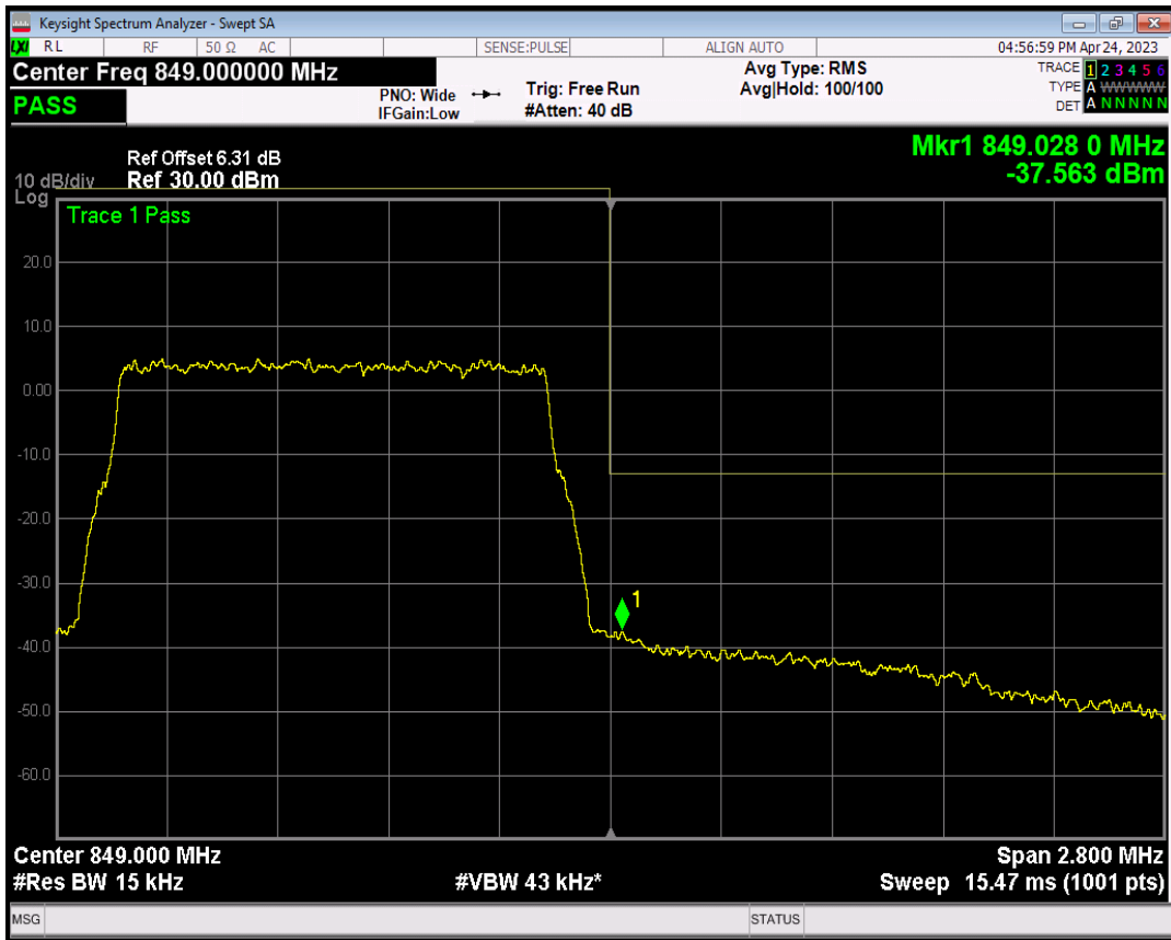
Band5 QPSK BW=3MHz Channel=20415 RB Size=1 Position=#0
