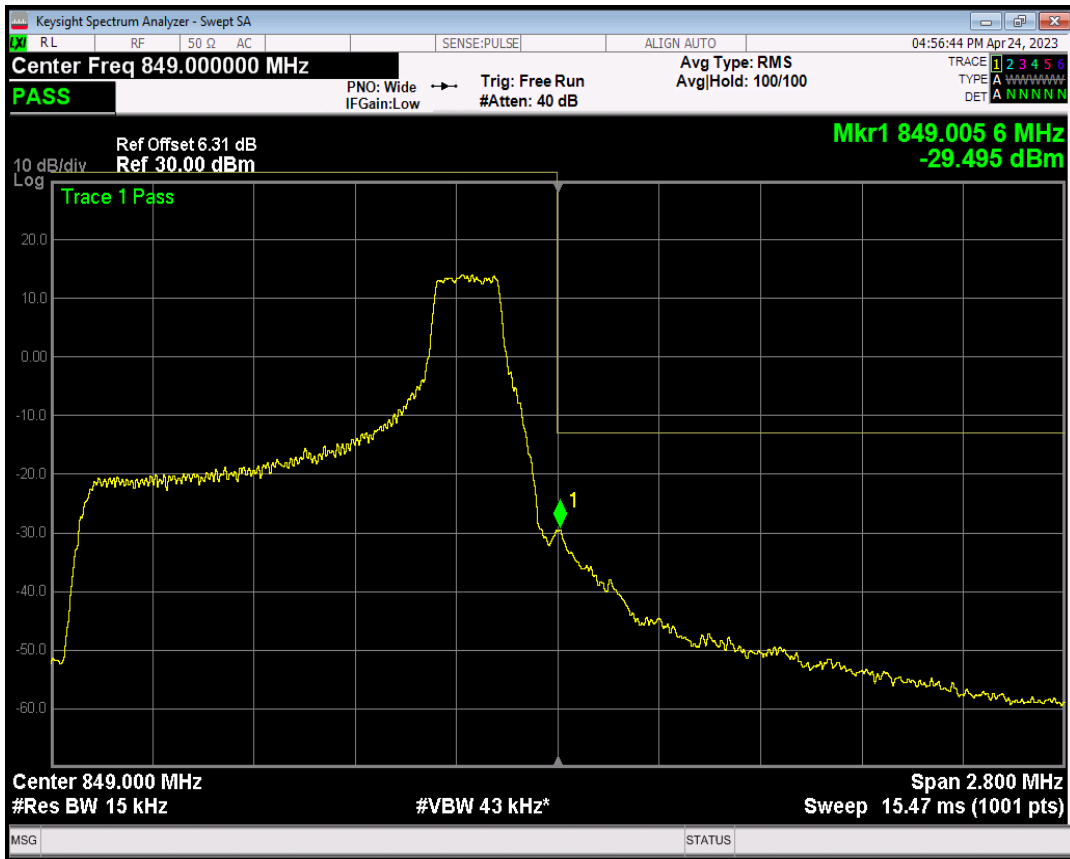
Band5 QPSK BW=1.4MHz Channel=20643 RB Size=6 Position=#0
