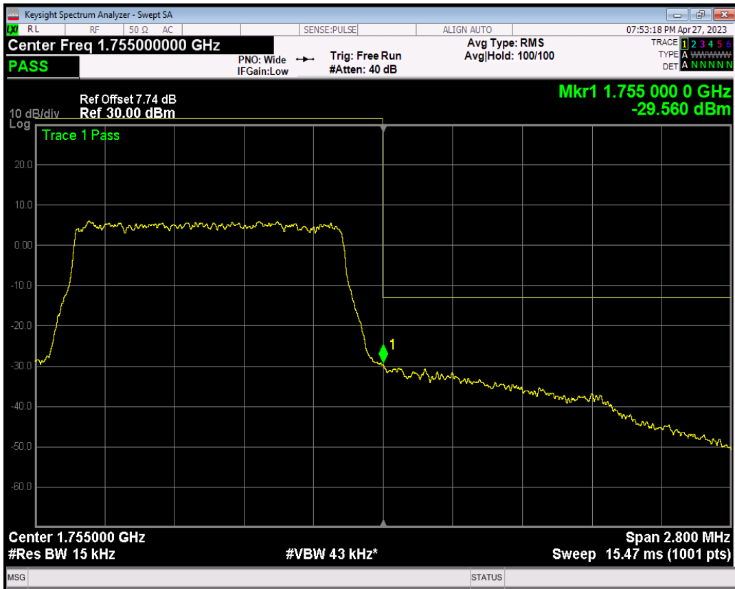
Band4 QPSK BW=1.4MHz Channel=20393 RB Size=6 Position=#0
