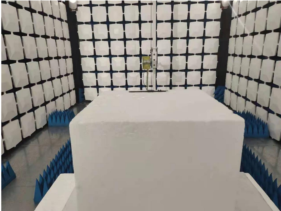
Above 1GHz for radiated emission test setup
