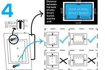
Push all the wires back into the wall box and try to allow as much space for the switch as possible.
