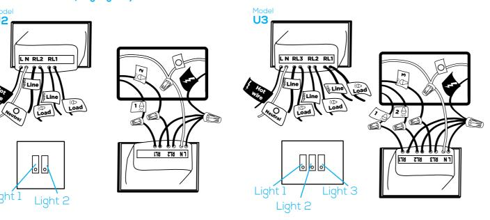
Input L/N should be connected to a 16A circuit breaker, and each way output should be connected to a 5A circuit breaker before used.
