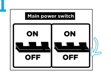
Turn off the power at the circuit breaker for the switch you are replacing.
