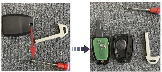
**Step3**: Now the key is opened. We can easily see the label here. The label is marked by a laser. This procedure is also the process of changing the battery
