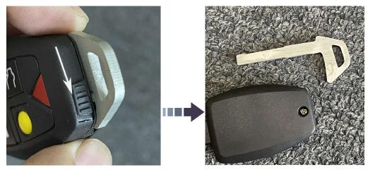
Step 2: Use a screwdriver to unscrew the screw and open the shell
