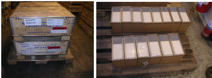
Shown above: different ways to correctly store monoblocs
