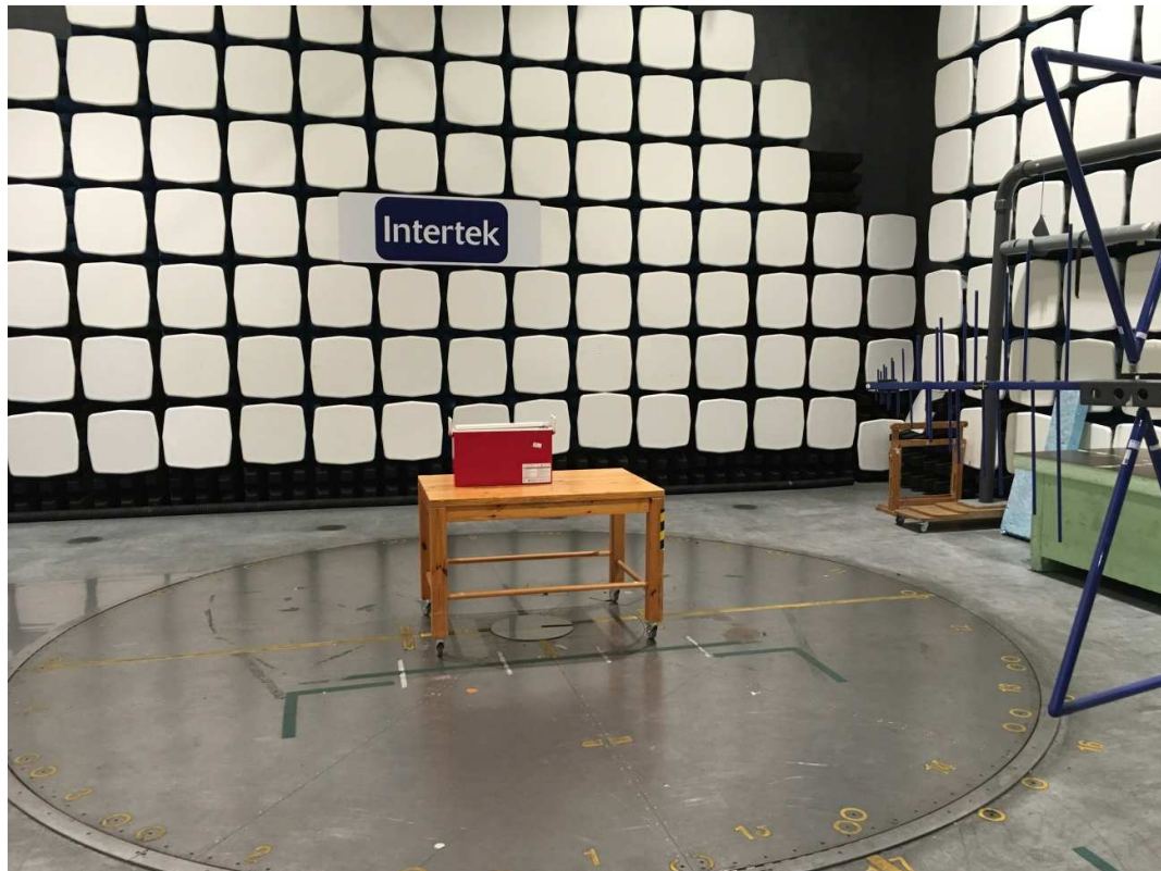
Test set up radiated emission 30 MHz – 1GHz
