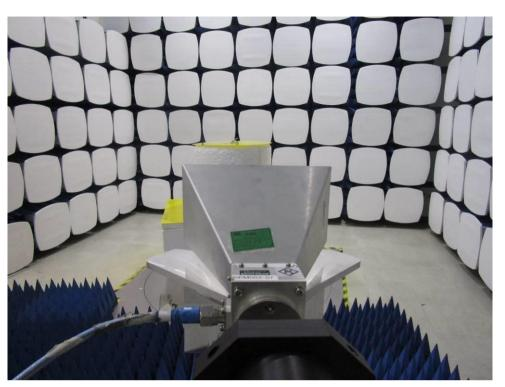
**1.3** Radiated Emissions which fall in the restricted bands Test Setup
