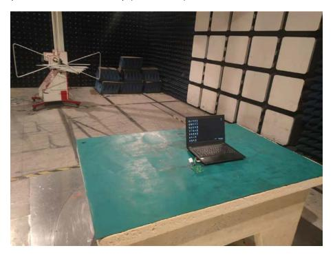
Spurious Emission Test Setup (Above 1GHz)
