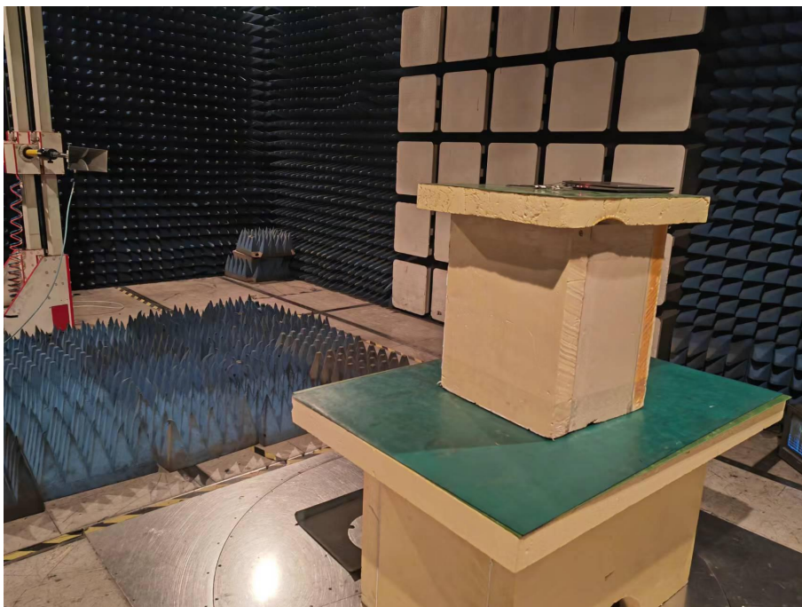
Spurious Emission Test Setup (Above 1GHz)
