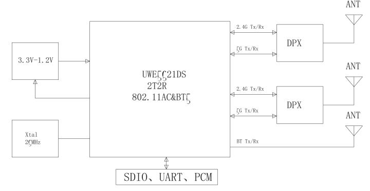
Figure 1 WF-U21DS-SSA1 Block Diagram
