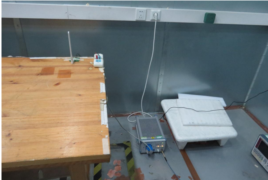
Picture 3 Conducted Emission Test Setup
