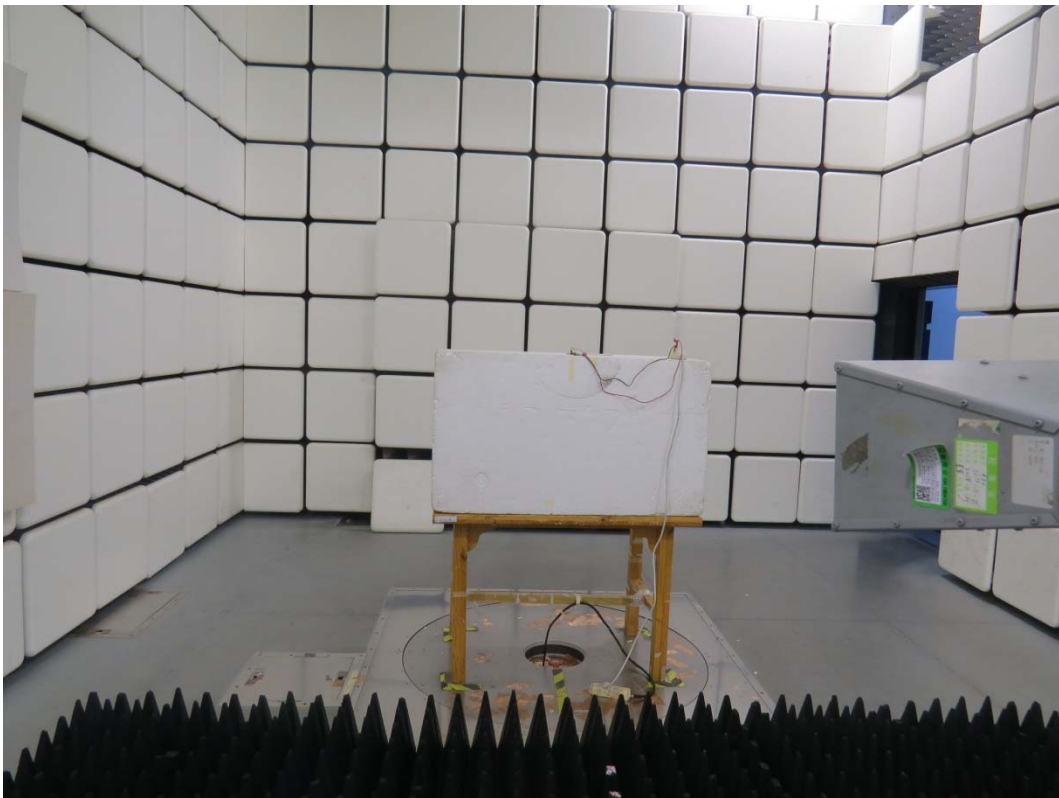
Picture 2 Radiated Spurious Emissions Test setup
