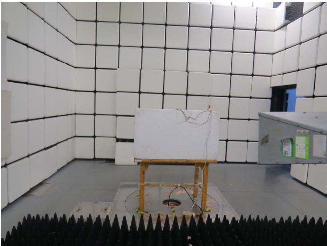
Picture 2 Radiated Spurious Emissions Test setup
