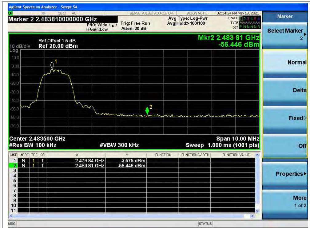
(Band edge, Channel 78, \pi/4 -DQPSK)
