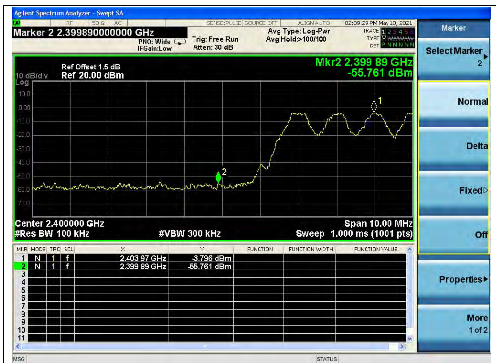
(Band edge with hopping on, Channel 0, GFSK)
