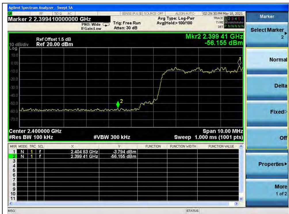
(Band edge with hopping on, Channel 0, 8-DPSK)
