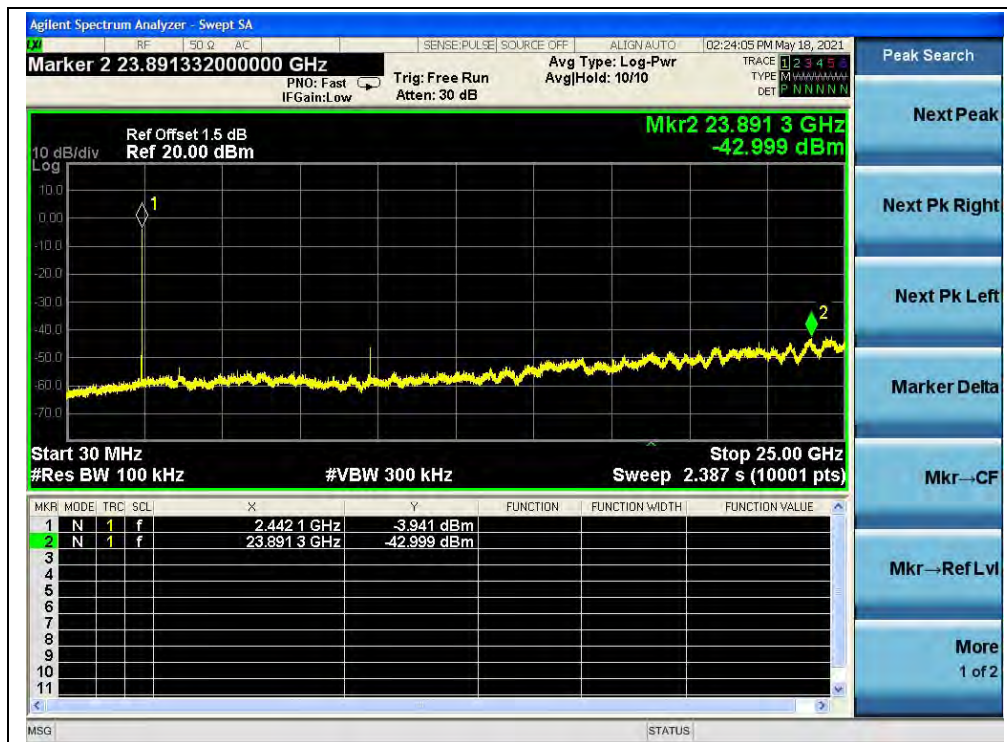
(30MHz to 25GHz, Channel 39, 8-DPSK)
