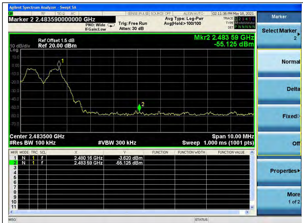
(Band edge with hopping on, Channel 78, GFSK)
