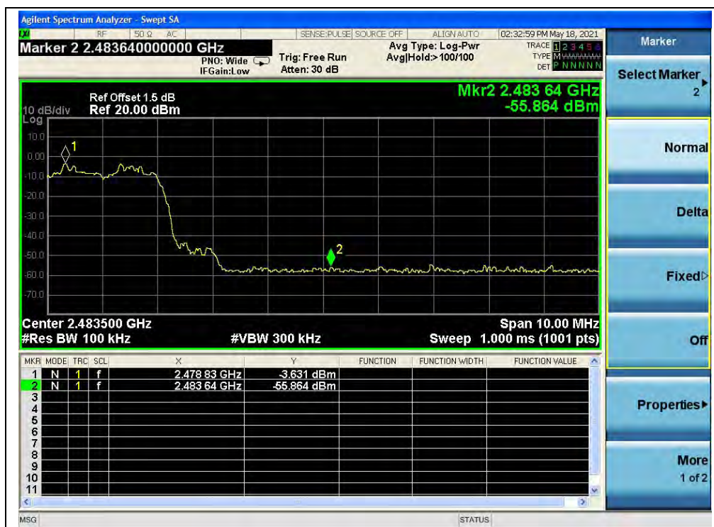
(Band edge with hopping on, Channel 78, 8-DPSK)
