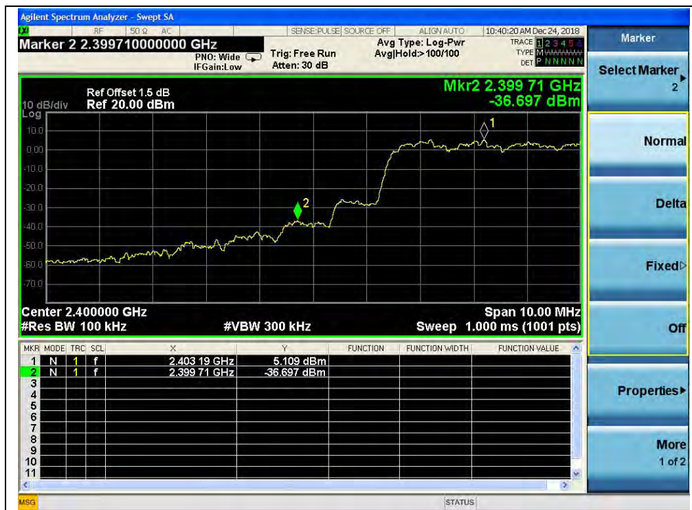
(Band edge with hopping on, Channel 0, 8-DPSK)
