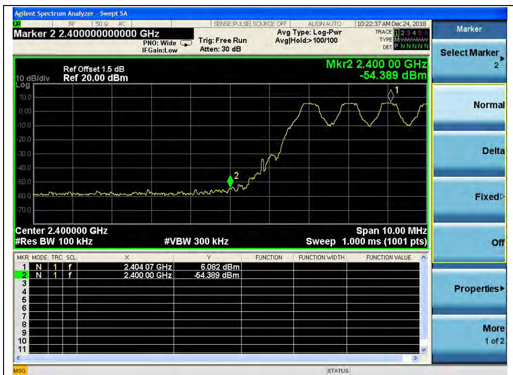
(Band edge with hopping on, Channel 0, GFSK)
