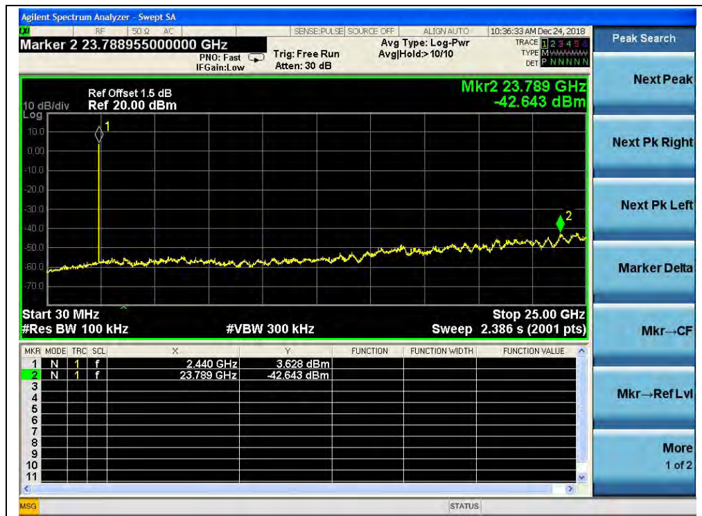
(30MHz to 25GHz, Channel 39, \pi/4 -DQPSK)
