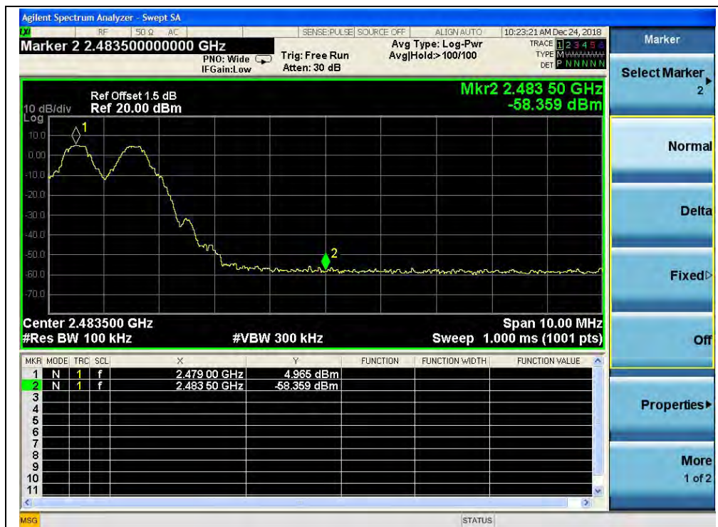
(Band edge with hopping on, Channel 78, GFSK)
