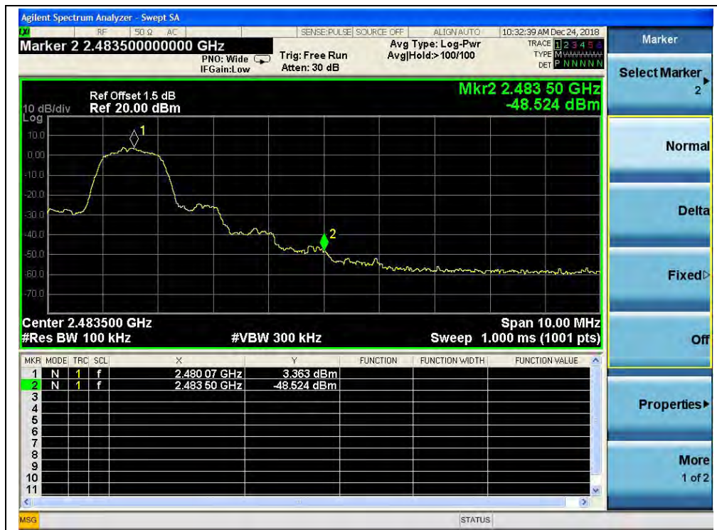
(Band edge, Channel 78, \pi/4 -DQPSK)
