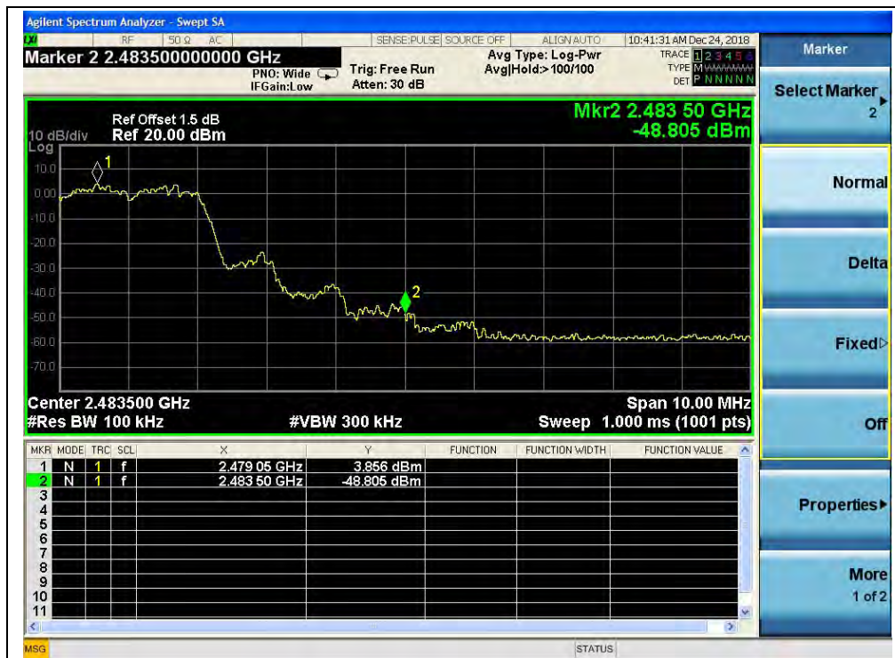
(Band edge with hopping on, Channel 78, 8-DPSK)
