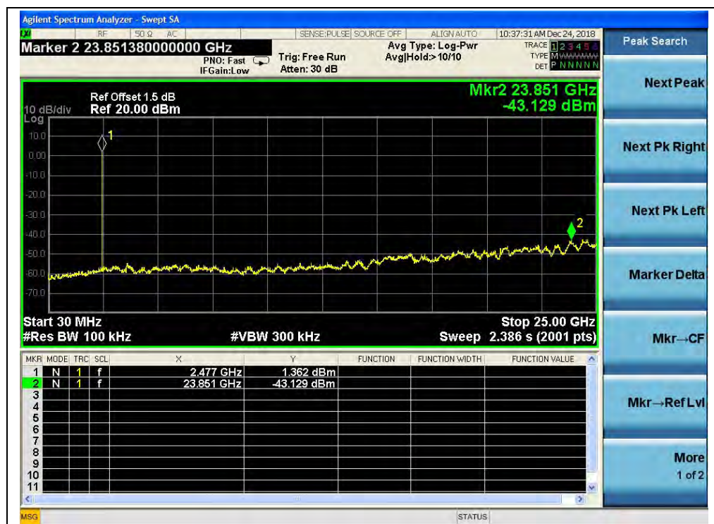
(30MHz to 25GHz, Channel 78, \pi/4 -DQPSK)
