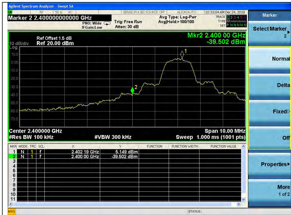
(Band edge, Channel 0, \pi/4 -DQPSK)
