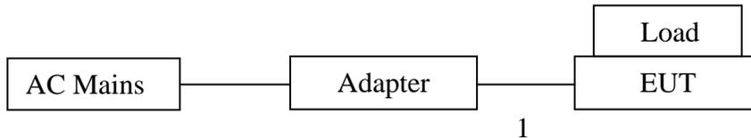
DC 5V From Adapter Input AC 120V/60Hz
