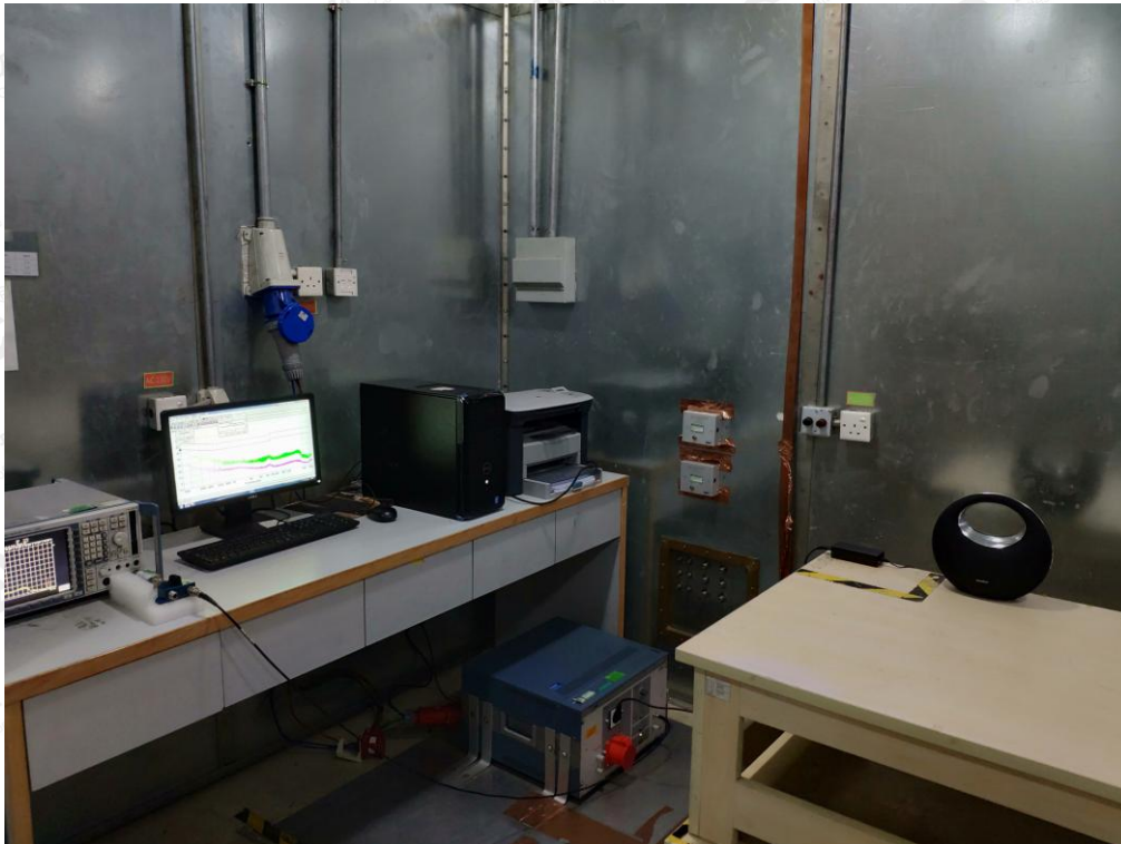
FCC RADIATED EMISSION TEST SETUP BELOW 1GHZ
