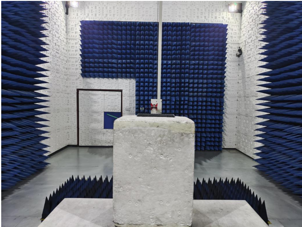
RADIATED EMISSION TEST SETUP ABOVE 1GHz
