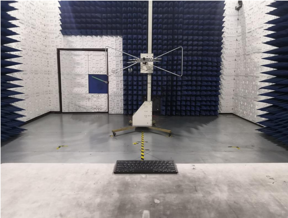
RADIATED EMISSION TEST SETUP ABOVE 1GHz
