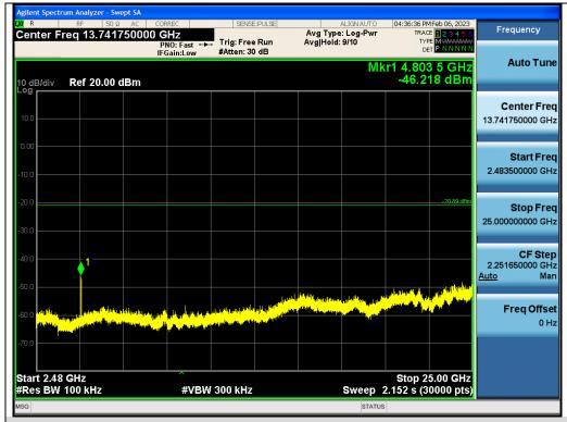
Test\_Graph\_LE1M\_ANT1\_2402\_1Mbps\_Higher Band Emissions
