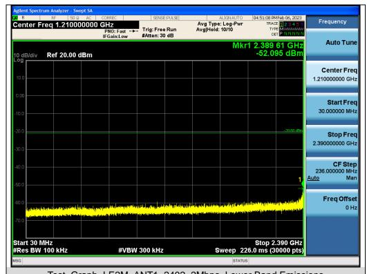
Test\_Graph\_LE2M\_ANT1\_2402\_2Mbps\_Lower Band Emissions
