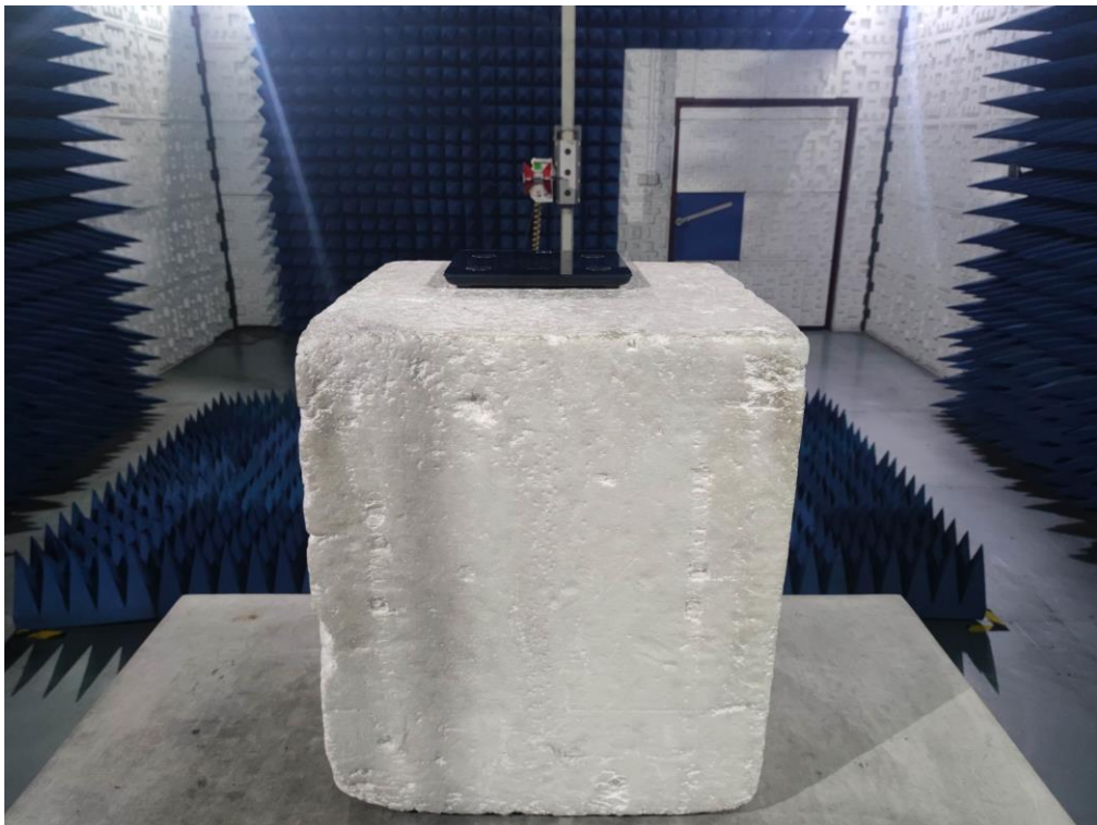
RADIATED EMISSION TEST SETUP ABOVE 1GHz
