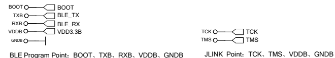
BLE Program Point: BOOT, TXB, RXB, VDD8, GND8 JLINK Point: TCK, TMS, VDD8, GND8
