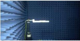
[Fig.2] DUT JIG(Quiet Zone 20Cm)
