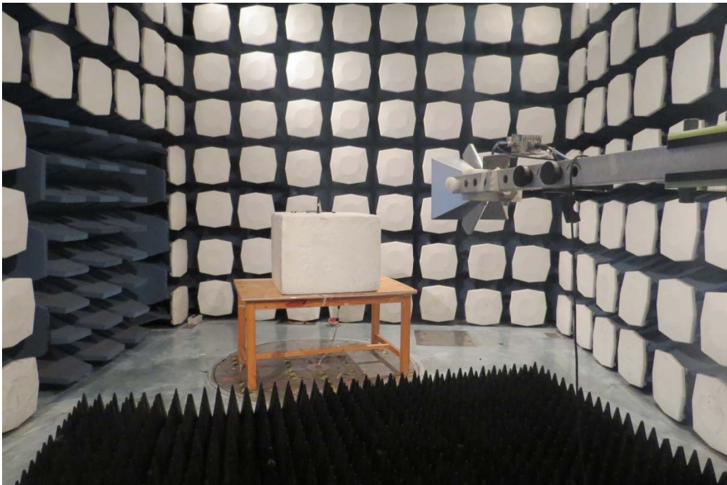
Picture 1: Radiated Spurious Emissions Test setup
