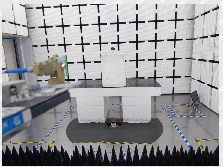
Radiation Emission Test Setup (Above 18GHz)
