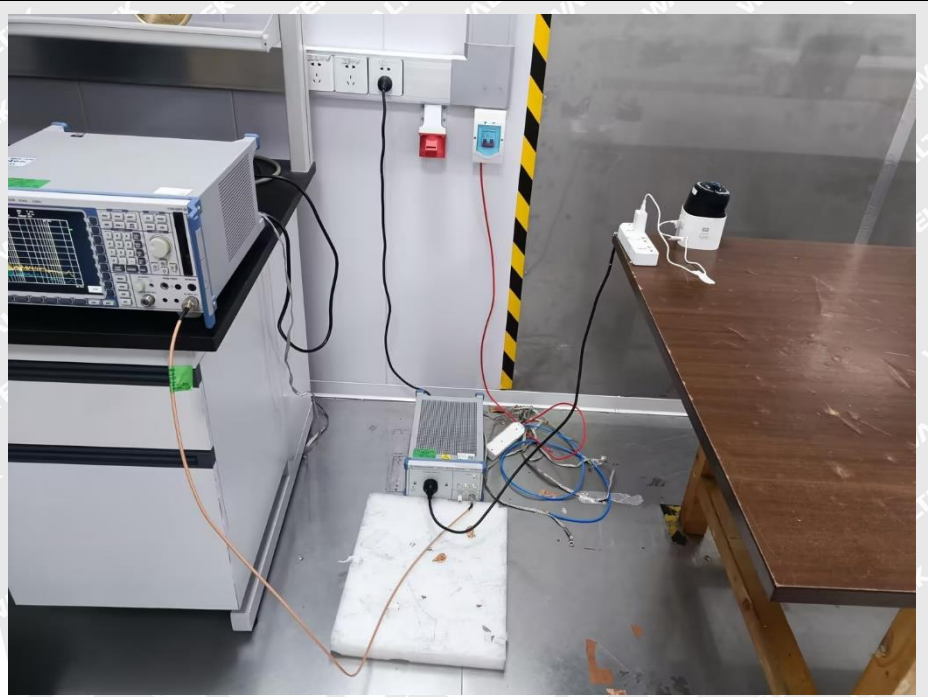
Conducted Emission Test Setup
