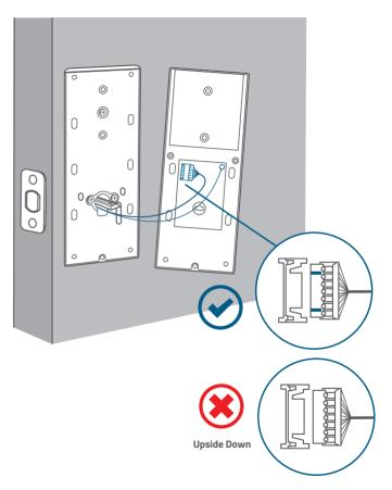
6. Mount the interior assembly. Make sure both wires are tucked into the cabin on the back of the interior assembly.
