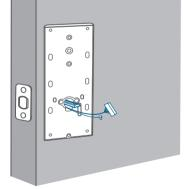
2. Run the wires through the back cover.
