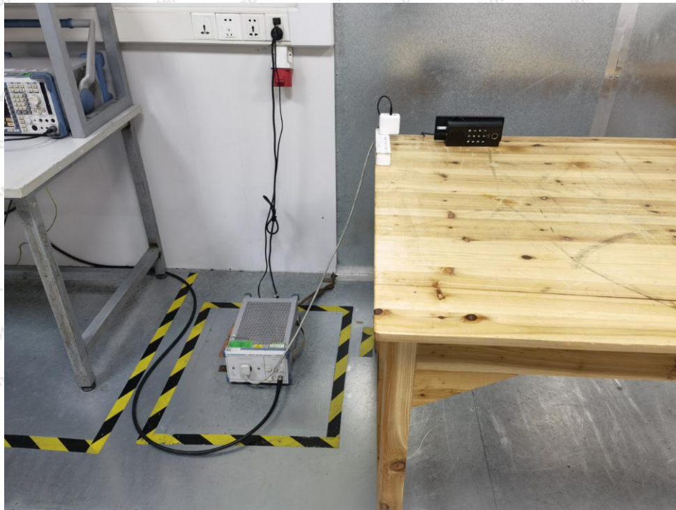
Photo of Conducted Emission Measurement
