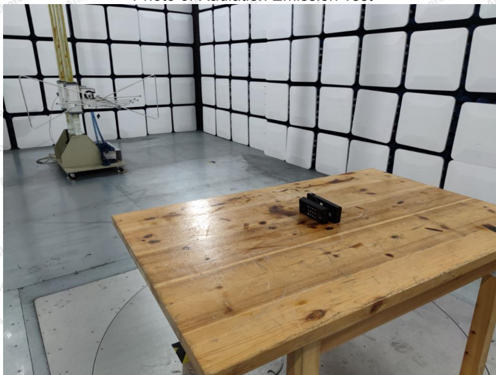
Photo of Radiation Emission Test
